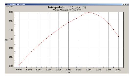
This figure shows the interpolated field strength perpendicular to the dipole. The interpolated points follow the raw points with no inconsistencies.
