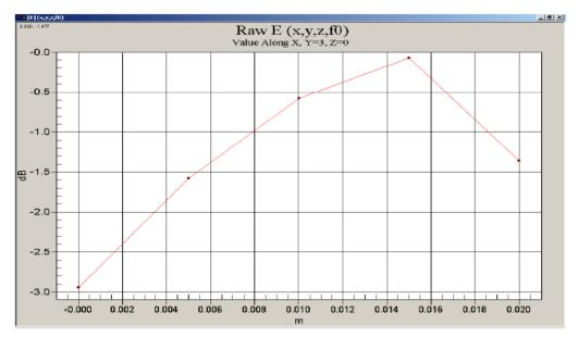
The figure above shows the raw measured field strength perpendicular to the length of the validation dipole. The TCB guidance slides require the 3dB width to be much larger than the step size. The width between -3dB points is  $\geq 21$ mm, at least 4 times the step size.
