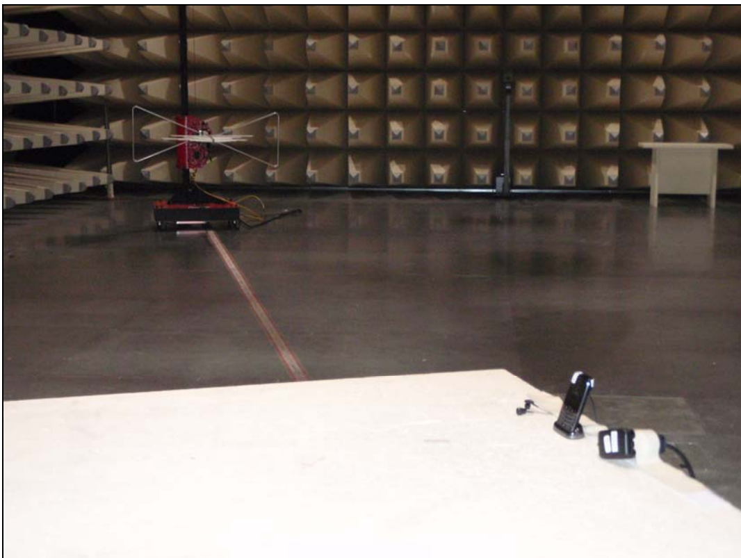
Photo 9: setup of radiated emission 30MHz – 1GHz (view to antenna)
