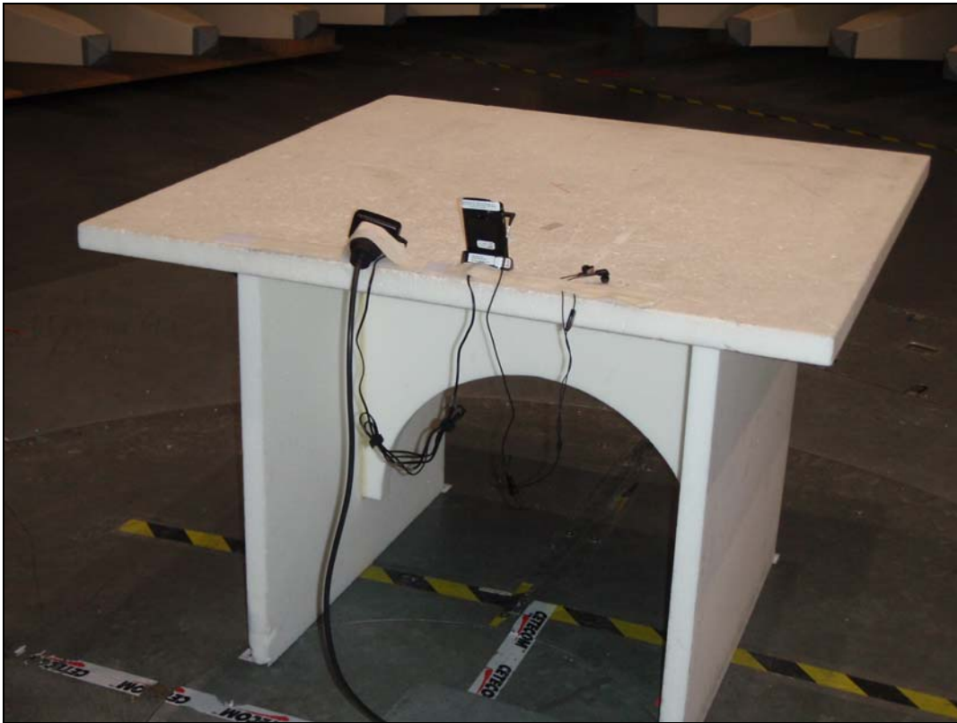
Photo 9: setup of radiated emission 30MHz – 1GHz (view to antenna)
