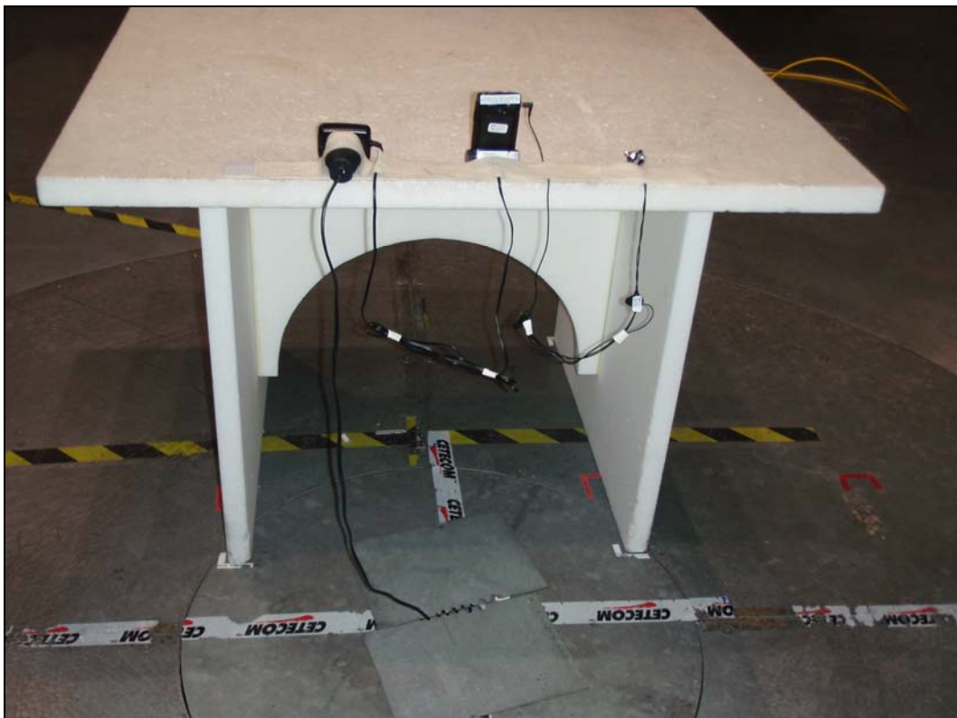
Photo 11: setup of radiated emission 1GHz – 10 GHz
