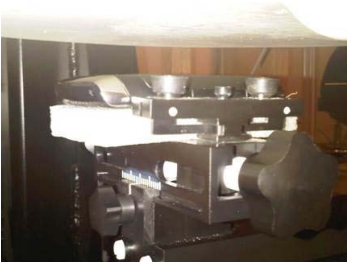
Figure E12. Body-worn configuration (No Holster, 25 mm away, back facing phantom)
