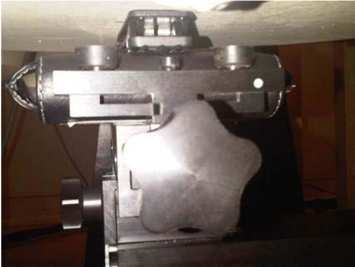
Figure E10. Body-worn configuration (Horizontal Holster, back facing phantom)
