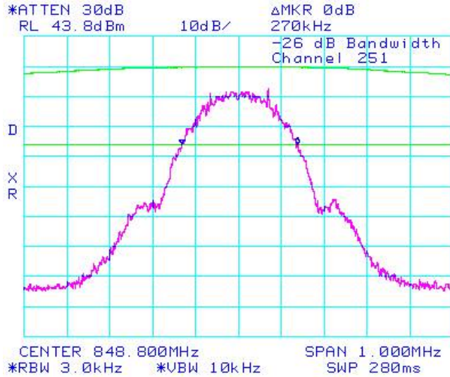
Figure 1-17a: -26dBc bandwidth, GSM850 band High Channel in GSM mode
