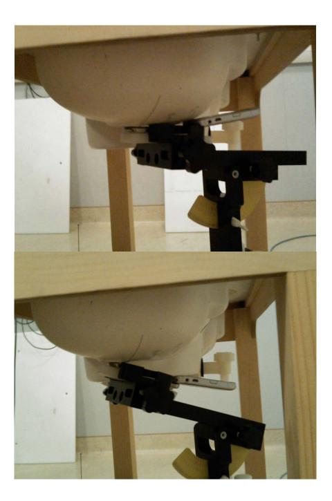
Figure E6. Head configuration (Right Touch/Tilt)
