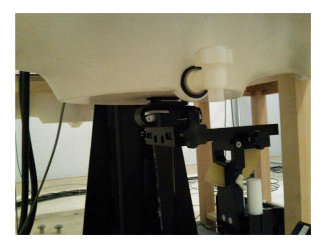
Figure E11. Body-worn configuration (Leather Holster, front facing phantom)
