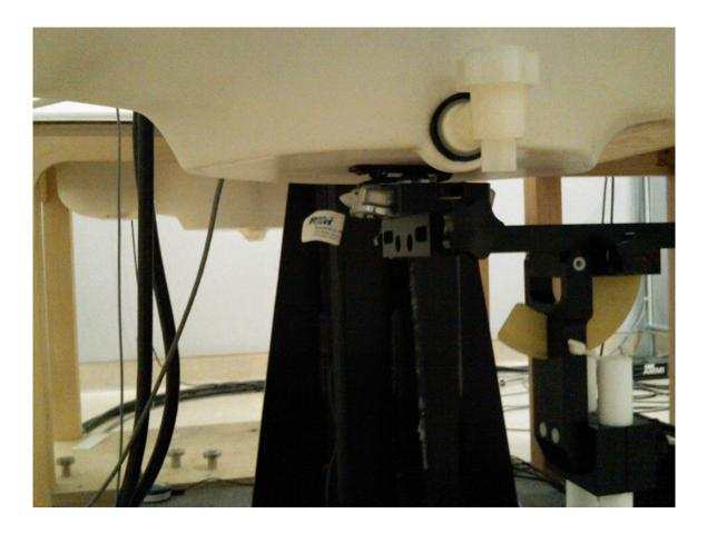
Figure E9. Body-worn configuration (Plastic Holster and headset, back facing phantom)
