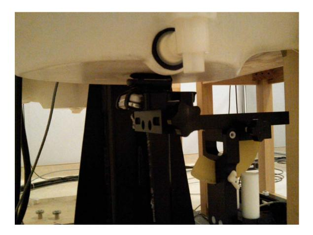
Figure E12. Body-worn configuration (Flip Holster, back facing phantom)
