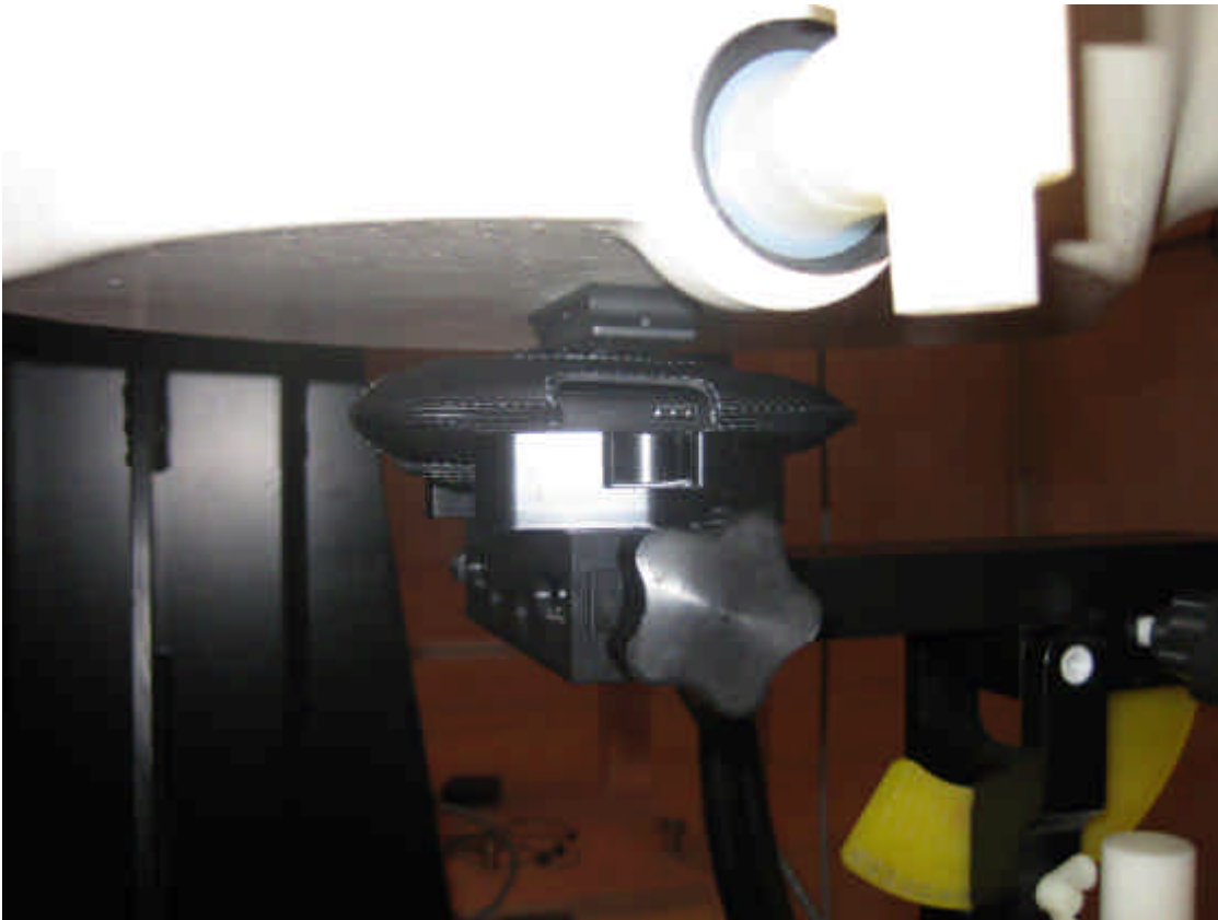
Figure E9. Body -worn configuration (Horizontal Holster, back facing phantom)
