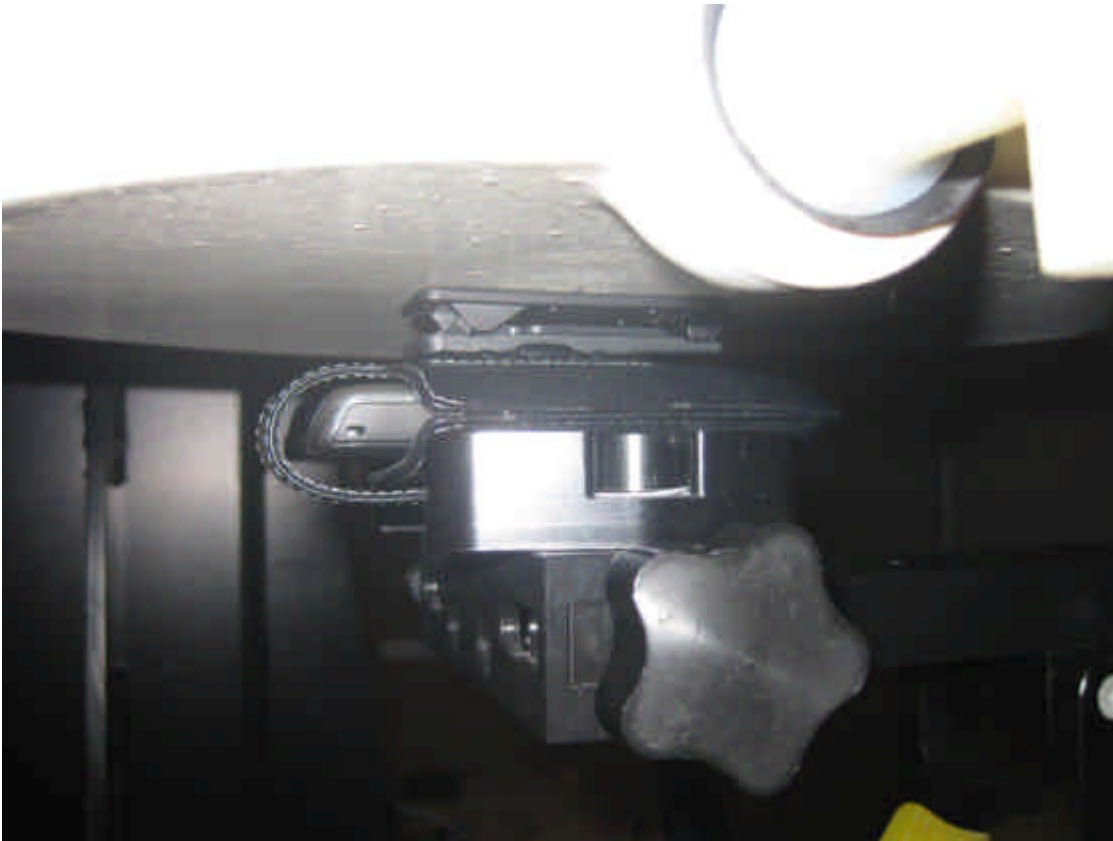
Figure E8. Body-worn configuration (Leather Swivel Holster, front facing phantom)
