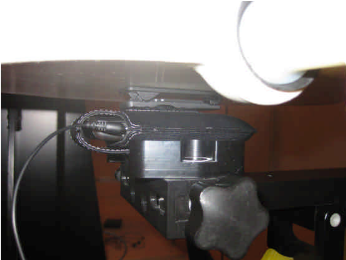
Figure E7. Body-worn configuration (Leather Swivel Holster , headset, back facing phantom)
