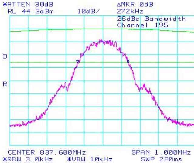
Figure 1-15: -26dBc bandwidth, GSM850 band Middle Channel in GSM mode
