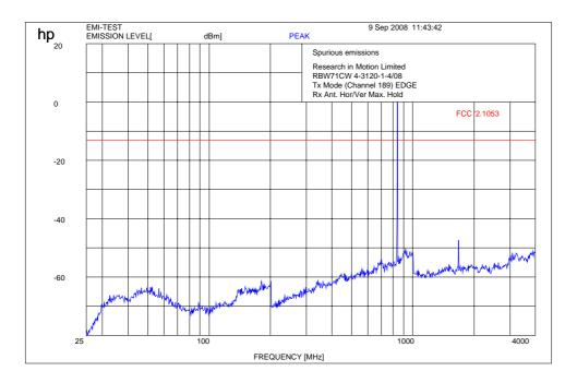
f < 1 GHz : RBW/VBW: 100 kHz The peak at 836 MHz shows the carrier  $f \geq 1GHz: RBW \ / \ VBW \ 1 \ MHz$
