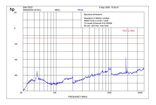
$\label{eq:general} \begin{array}{ll} f < 1 \ GHz: RBW/VBW: 100 \ kHz & f \geq 1 GHz: RBW \ / \ VBW \ 1 \ MHz \\ Carrier \ suppressed \ with \ a \ rejection \ filter \end{array}$
