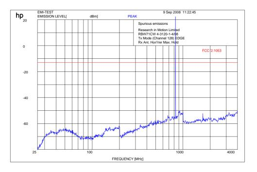
$f < 1 \ GHz$  : RBW/VBW: 100 kHz The peak at 824 MHz shows the carrier
