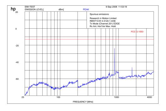
f < 1 GHz : RBW/VBW: 100 kHz The peak at 848 MHz shows the carrier  $f \geq 1 GHz: RBW \ / \ VBW \ 1 \ MHz$
