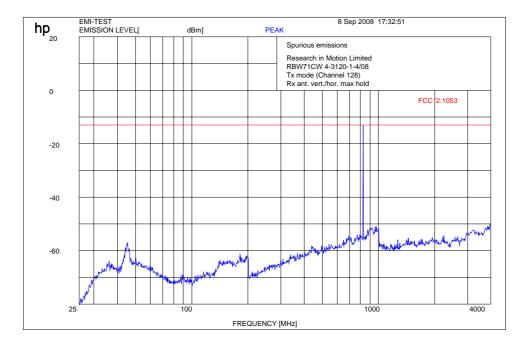
f < 1 GHz : RBW/VBW: 100 kHz The peak at 824 MHz shows the carrier  $f \geq 1 GHz: RBW \ / \ VBW \ 1 \ MHz$
