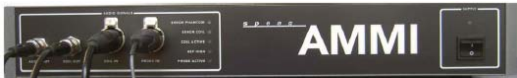
Figure 3: The Audio band Magnetic field Measuring Instrument (AMMI)
