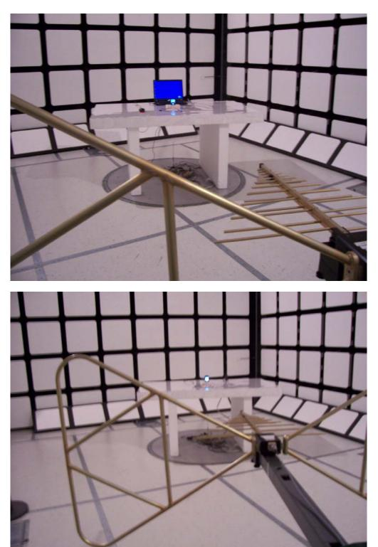
Radiated Emissions Test-Setup Photos
