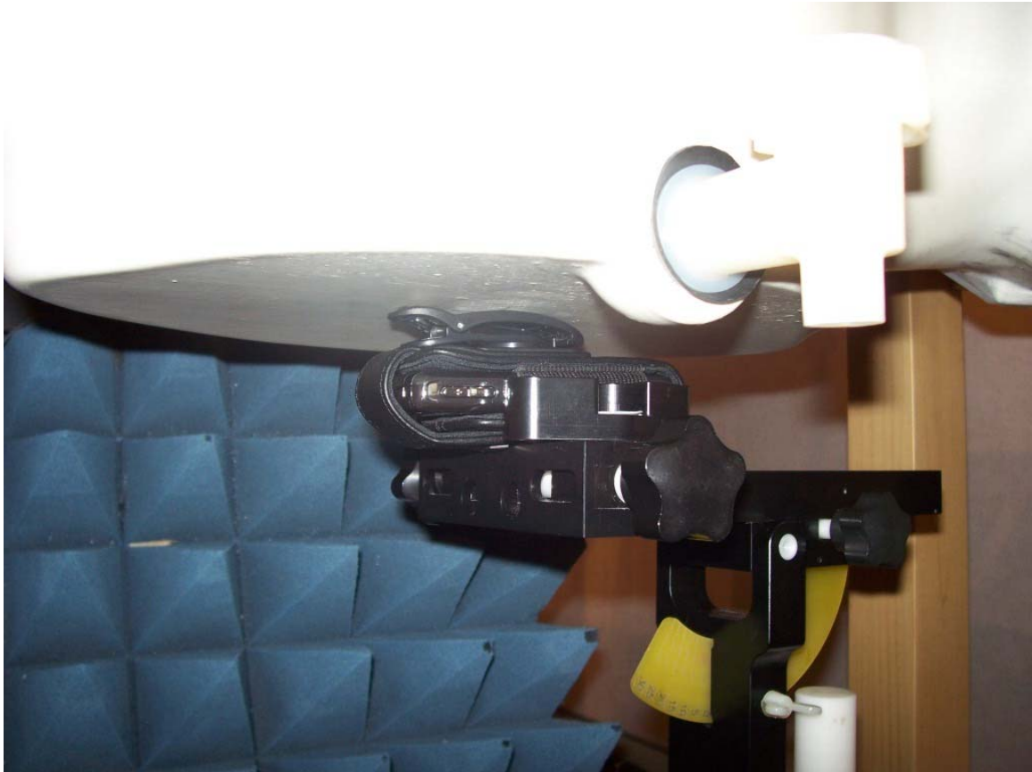
Figure E10. Body-worn configuration (Leather Holster, back facing phantom)
