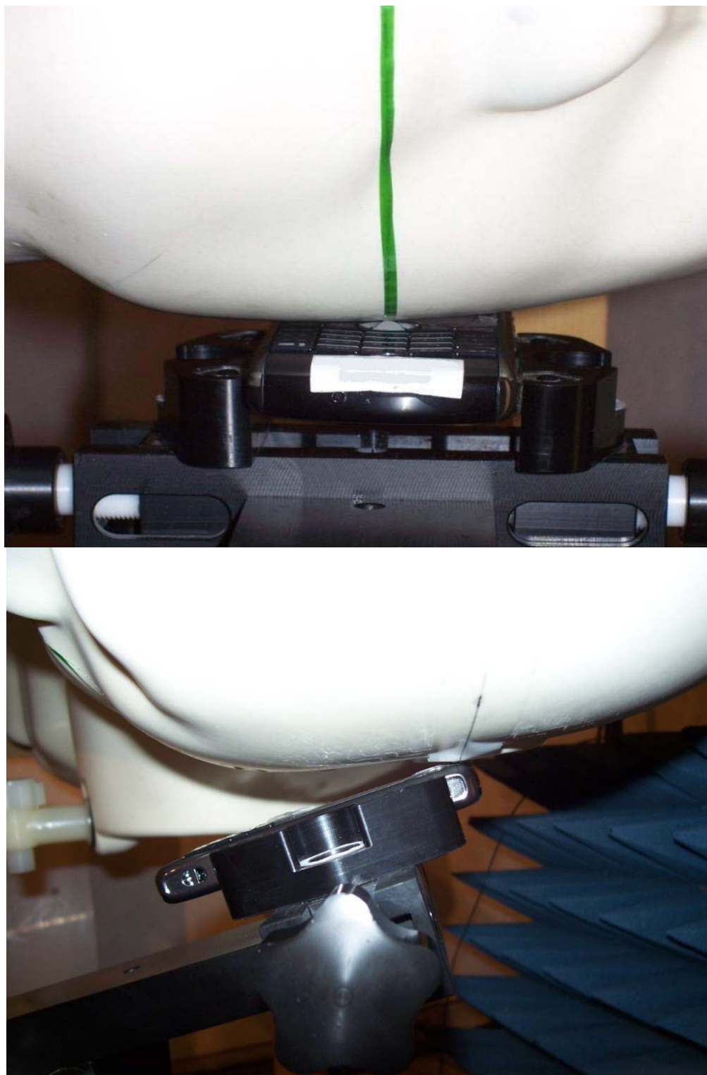
Figure E4. Head configuration (Left Touch/Tilt)
