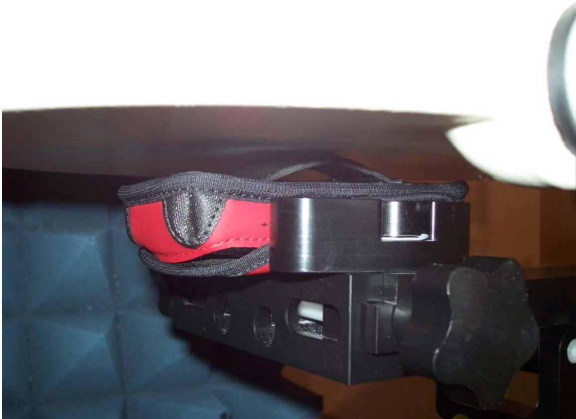
Figure E9. Body-worn configuration (Sports case without clip or strap, back facing phantom)
