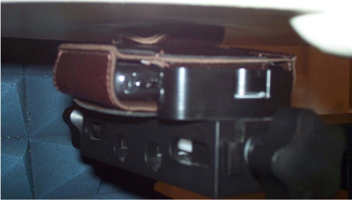
Figure E6. Body-worn configuration (Horizontal Holster, back facing phantom)
