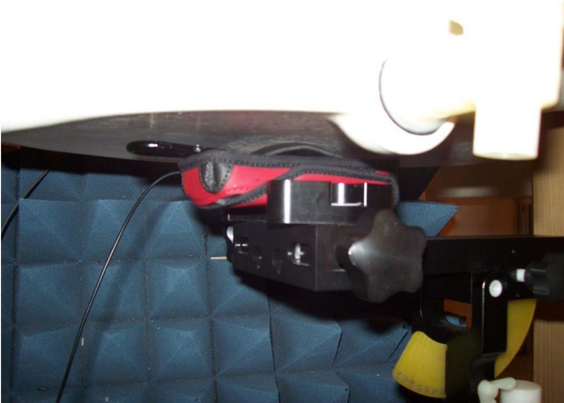
Figure E14. Body-worn configuration (Sportscase with clip, headset and BT on, back facing phantom)
