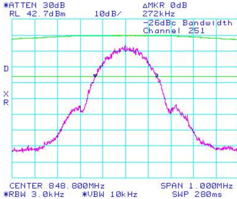
Figure 17: -26dBc bandwidth, GSM850 band High Channel in GSM mode
