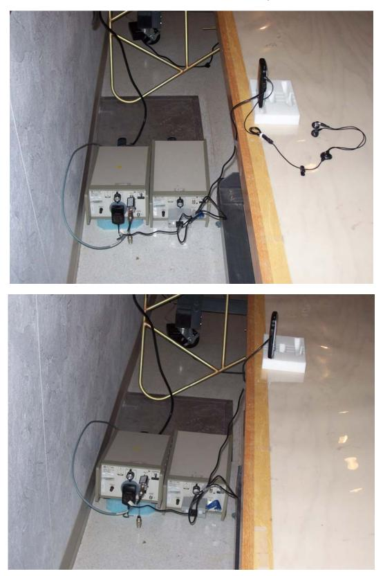
AC Line Conducted Emission Test-Setup Photos
