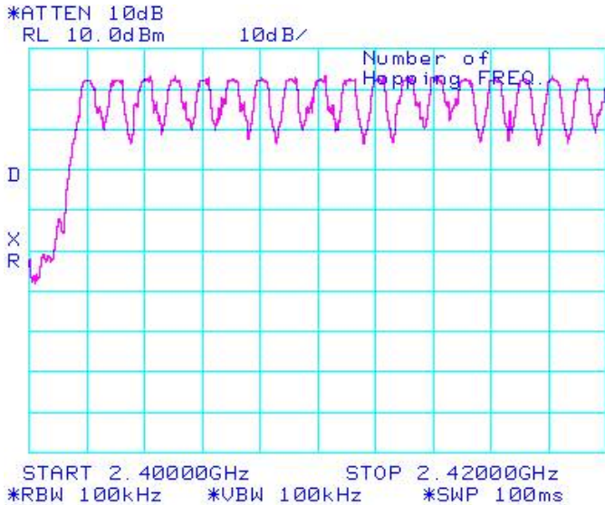
Figure 3-6: Number of Hopping Frequencies Static PBRs, DH5
