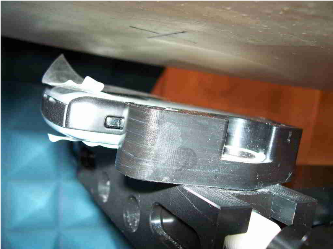
Figure E11. Body-worn configuration (No Holster, 25 mm away, back facing phantom)
