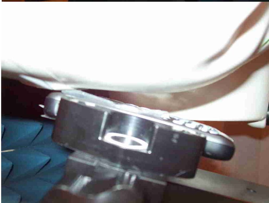
Figure E3. Head configuration (Right Touch/Tilt)
