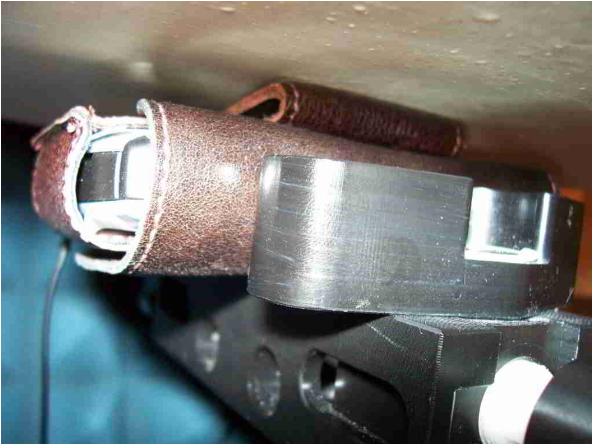
Figure E10. Body-worn configuration (Holster5, headset, back facing phantom)
