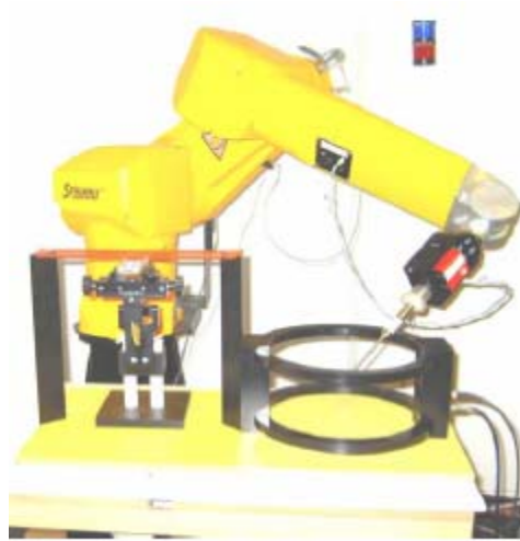
Figure 2: T-Coil set up with HAC Test Arch with Helmholtz Coil (AMCC)
