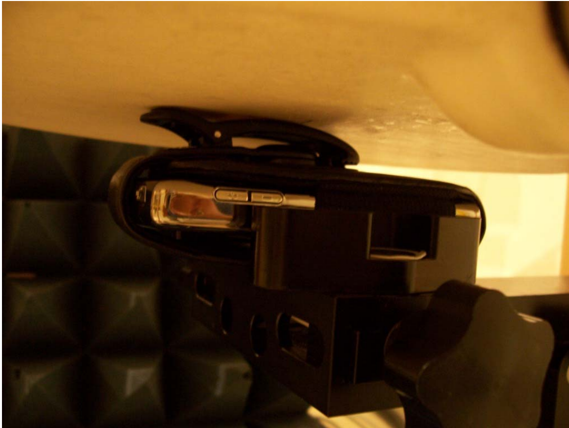
Figure E6. Body-worn configuration (Headset and Bluetooth connected, back facing phantom)
