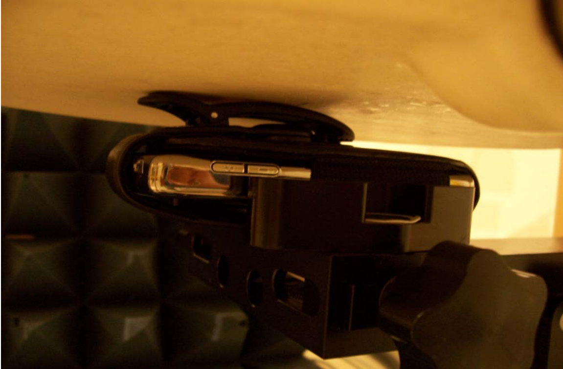
Figure E3. Body-worn configuration (Holster, back facing phantom)
