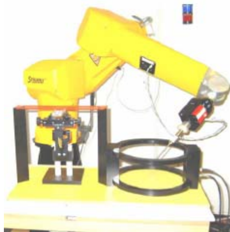
Figure 2: T-Coil set up with HAC Test Arch with Helmholtz Coil (AMCC)
