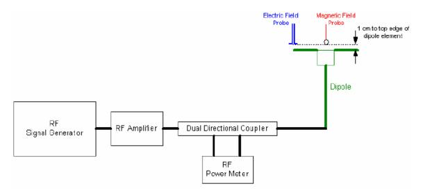
Figure 2: Dipole Validation Procedure
