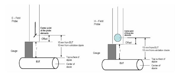
Figure 3: Gauge Block with E-Field & H-Field probes
