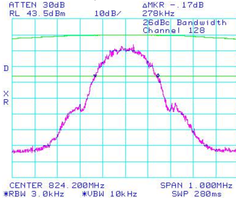
Figure 13: -26dBc bandwidth, GSM850 band Low Channel in GSM mode
