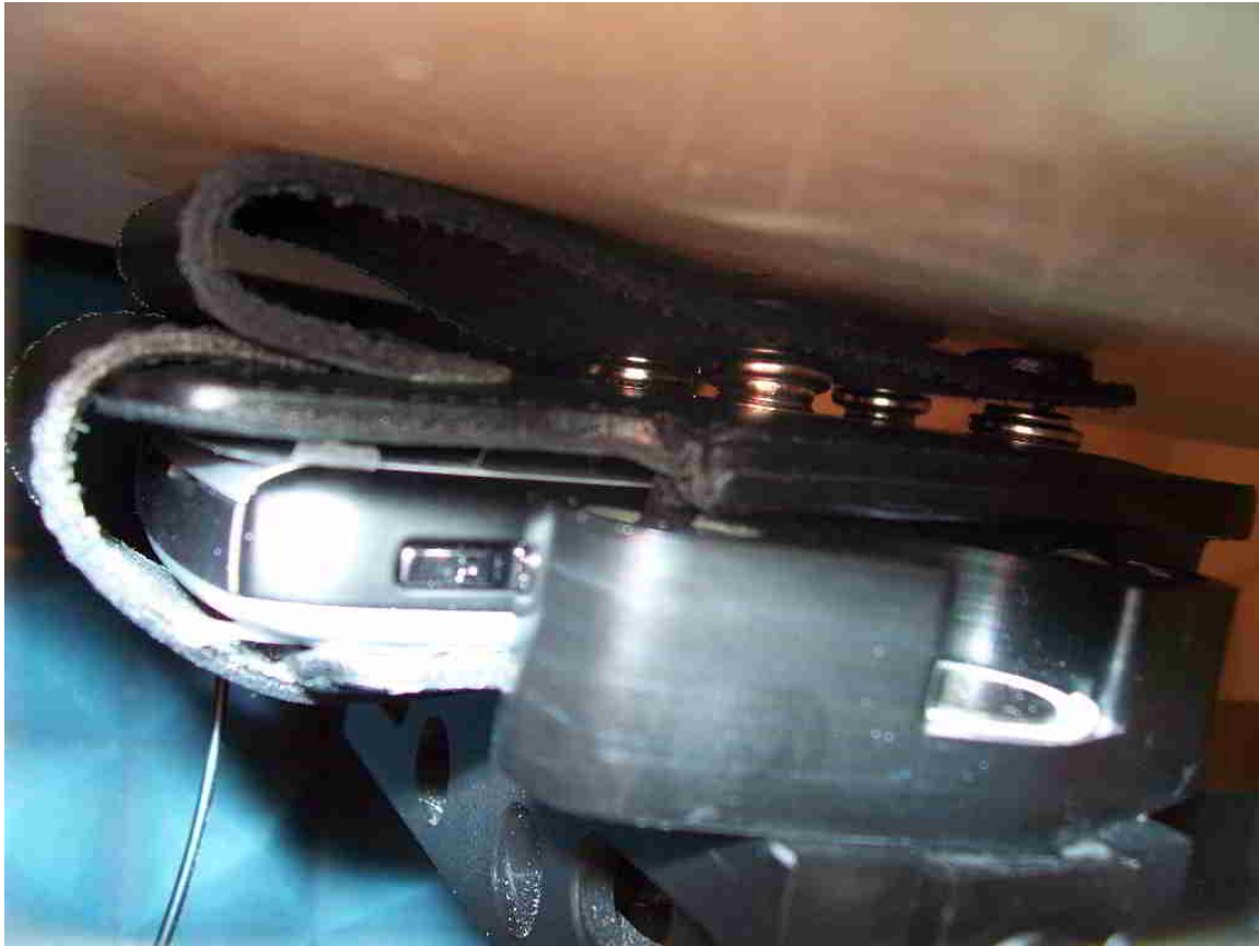
Figure E8. Body-worn configuration (Holster6, headset, back facing phantom)
