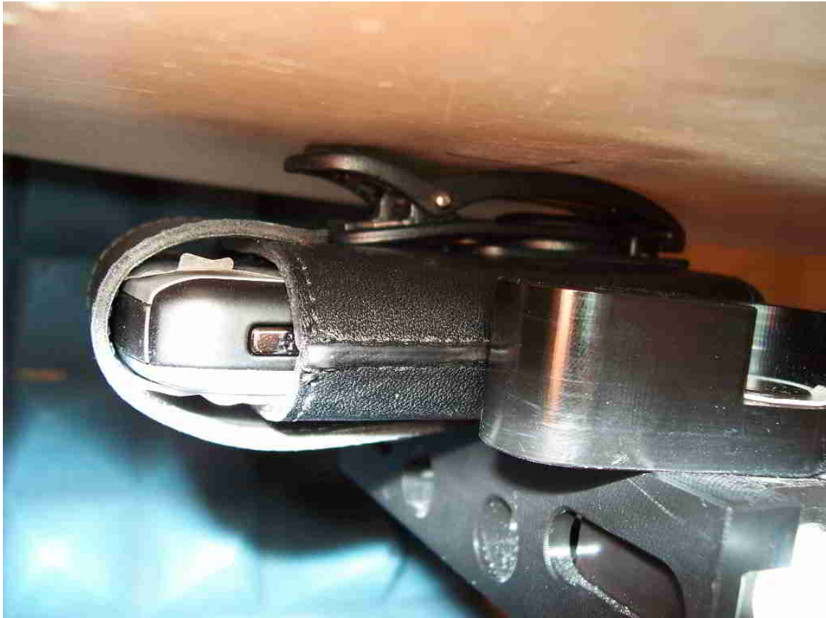
Figure E6. Body-worn configuration (Holster4, back facing phantom)
