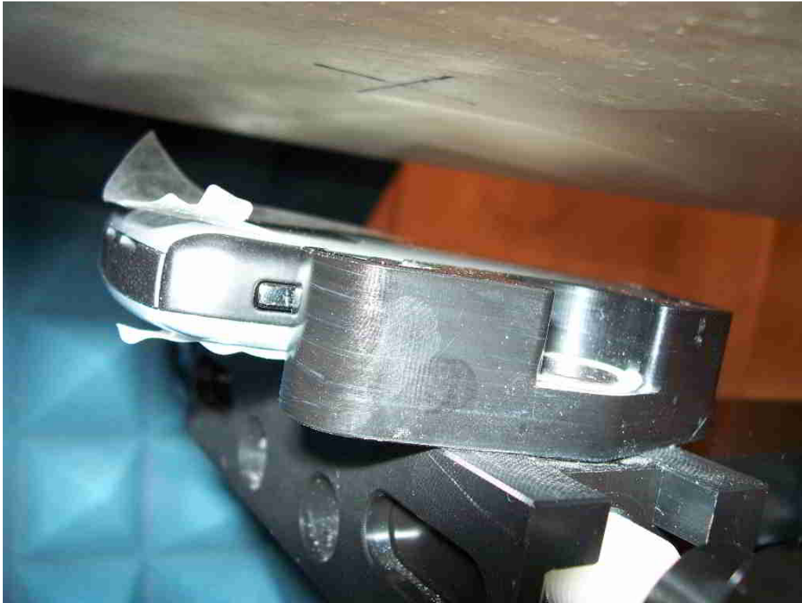
Figure E9. Body-worn configuration (No Holster, 25 mm away, back facing phantom)
