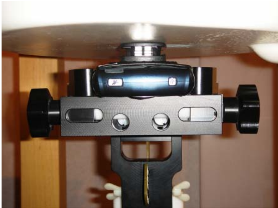
Figure E2. Body worn configuration (Plastic Holster; Front side facing phantom)
