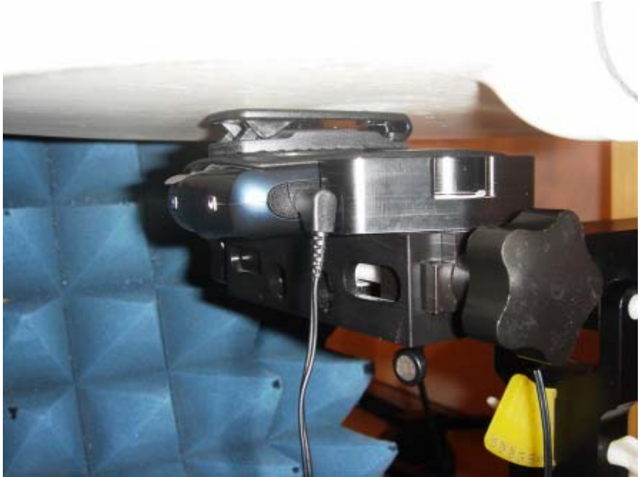
Figure E4. Body worn configuration (Plastic Holster; Headset and Bluetooth connected; Front side facing phantom)
