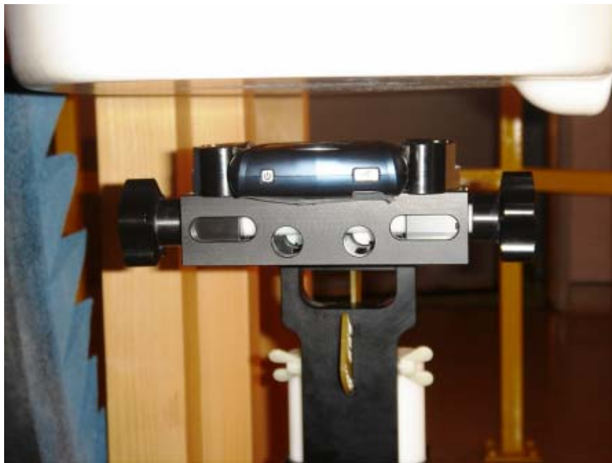
Figure E3. Body worn configuration (No Holster; 25 mm away; Back side facing phantom)
