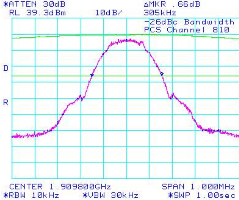
Figure 23: -26dBc bandwidth, PCS High Channel
