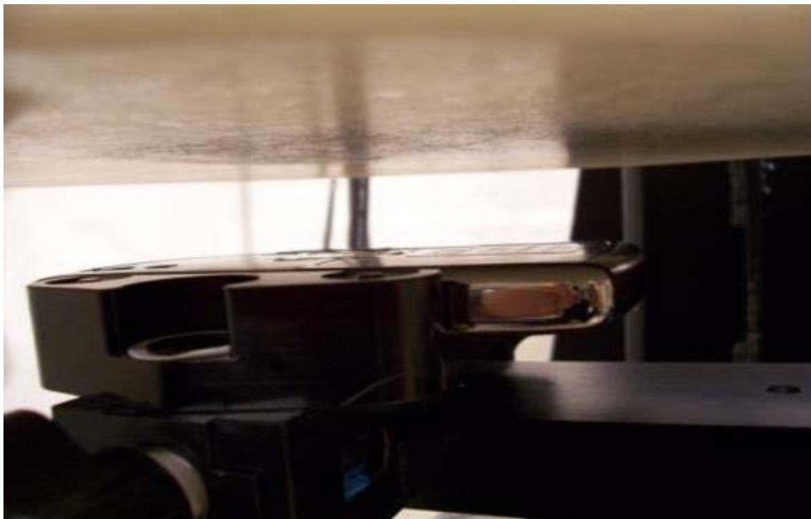
Figure E5. Body-worn configuration (No Holster, 25 mm away, back facing phantom)
