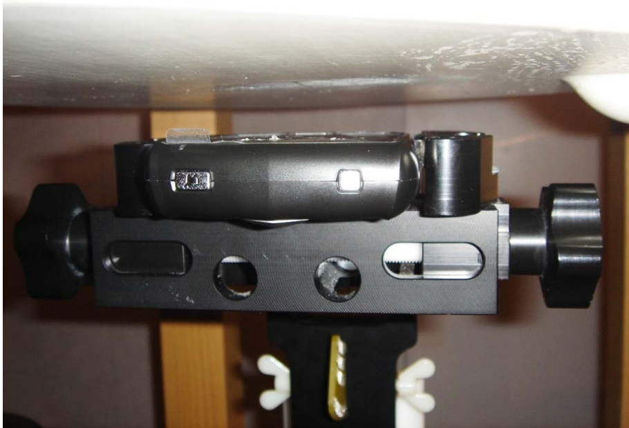
Figure E13. Body-worn configuration (No Holster, 15 mm away, front facing phantom)
