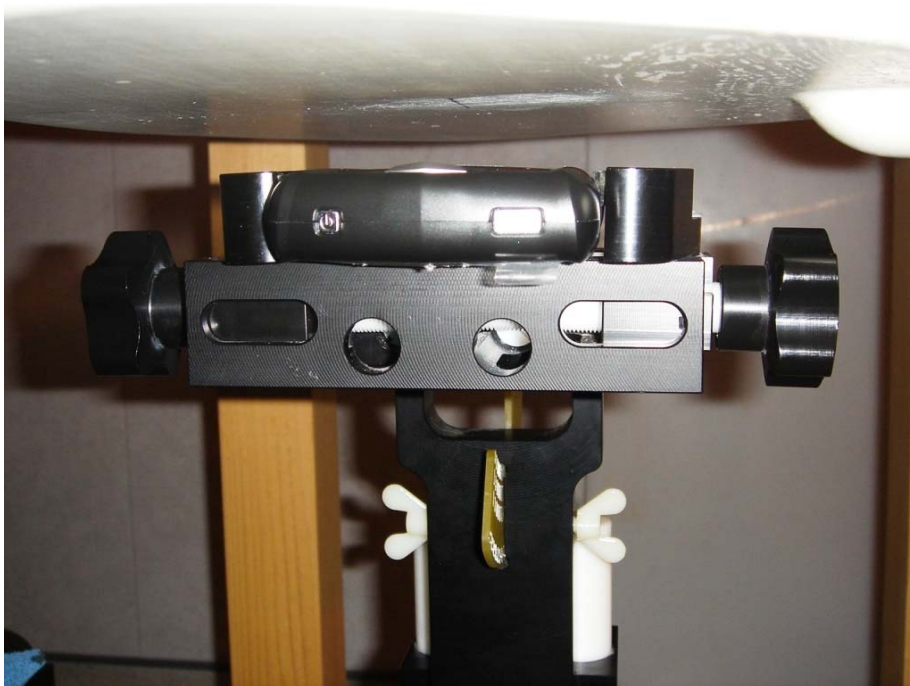
Figure E14. Body-worn configuration (No Holster, 15 mm away, back facing phantom)
