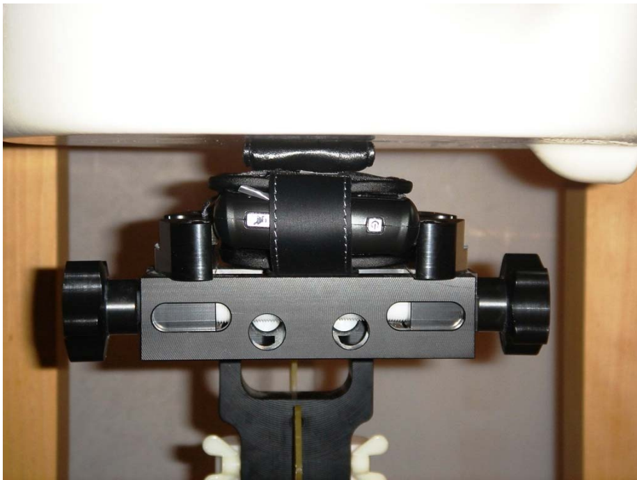
Figure E11. Body-worn configuration (Leather Holster 4, front facing phantom)
