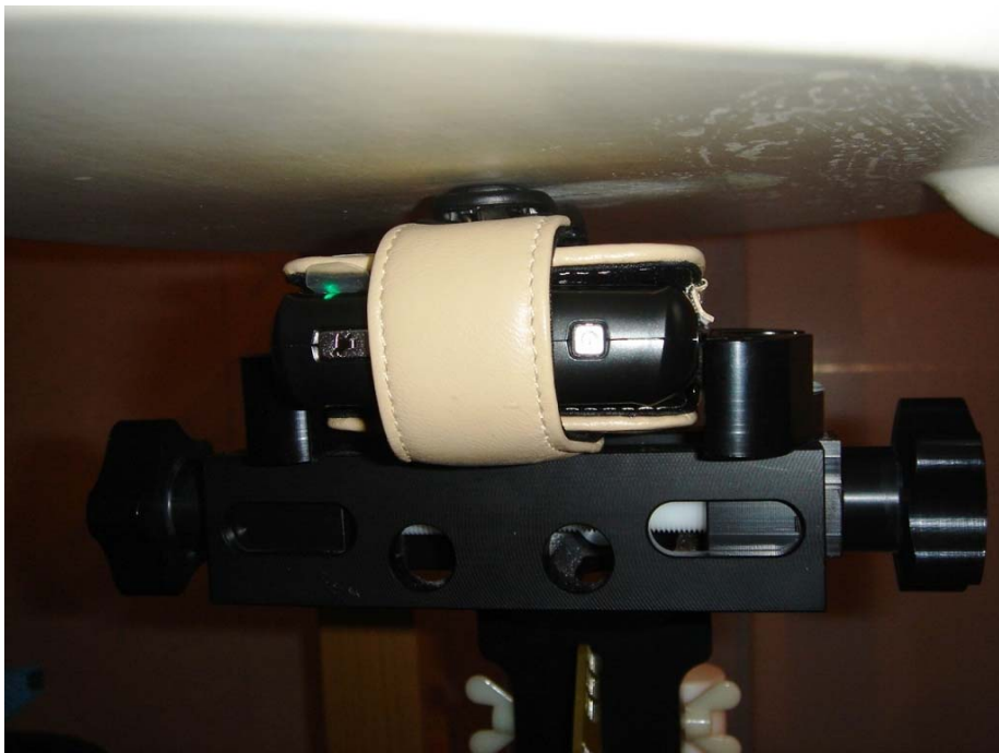
Figure E9. Body-worn configuration (Leather Holster 2, front facing phantom)
