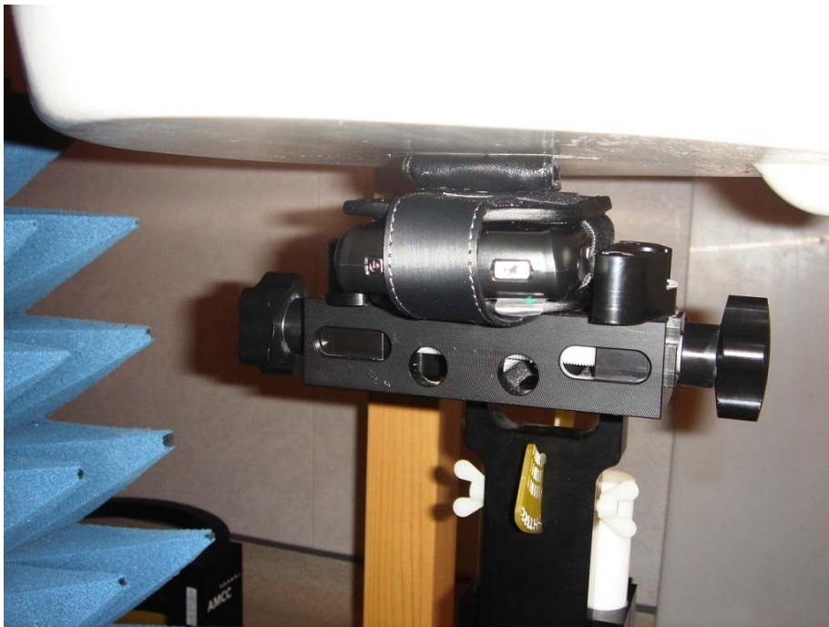
Figure E12. Body-worn configuration (Leather Holster 4, back facing phantom)
