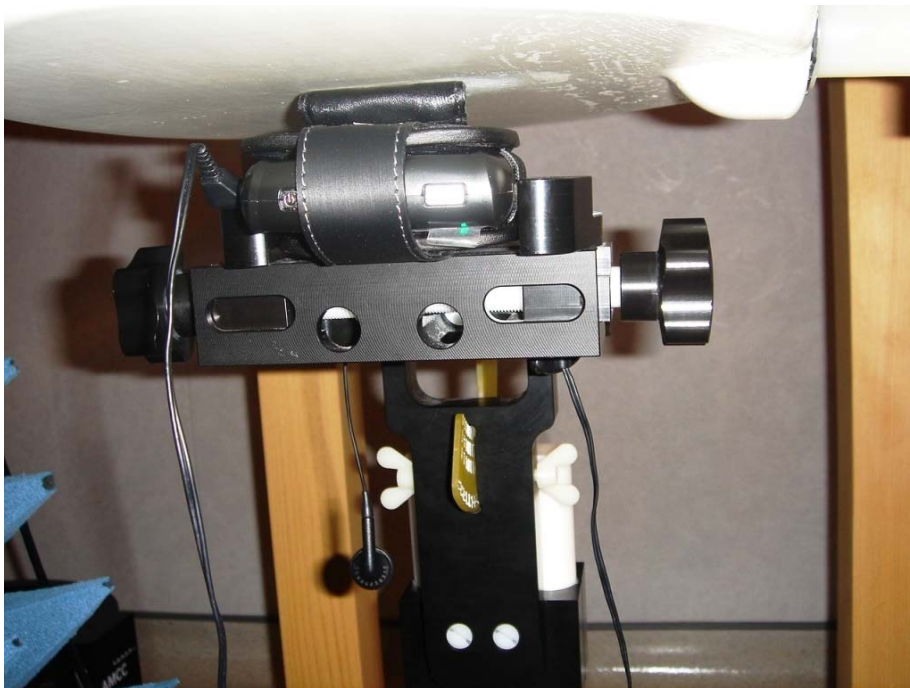
Figure E16. Body-worn configuration (Leather Holster 4, back facing phantom, headset attached)
