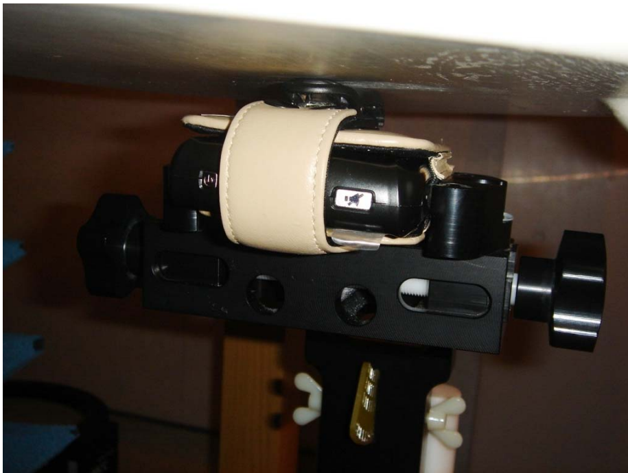
Figure E10. Body-worn configuration (Leather Holster 2, back facing phantom)
