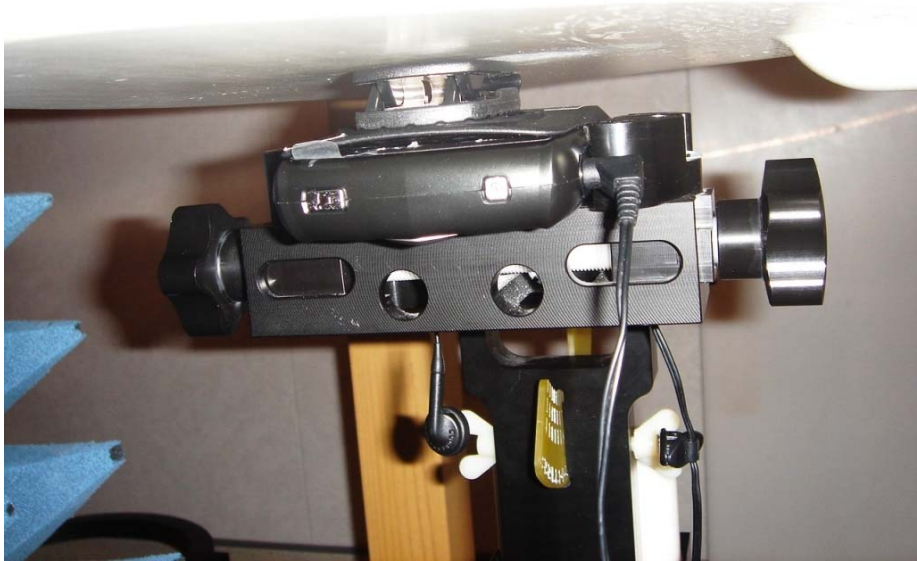
Figure E15. Body-worn configuration (Plastic Holster 1, front facing phantom, headset attached)
