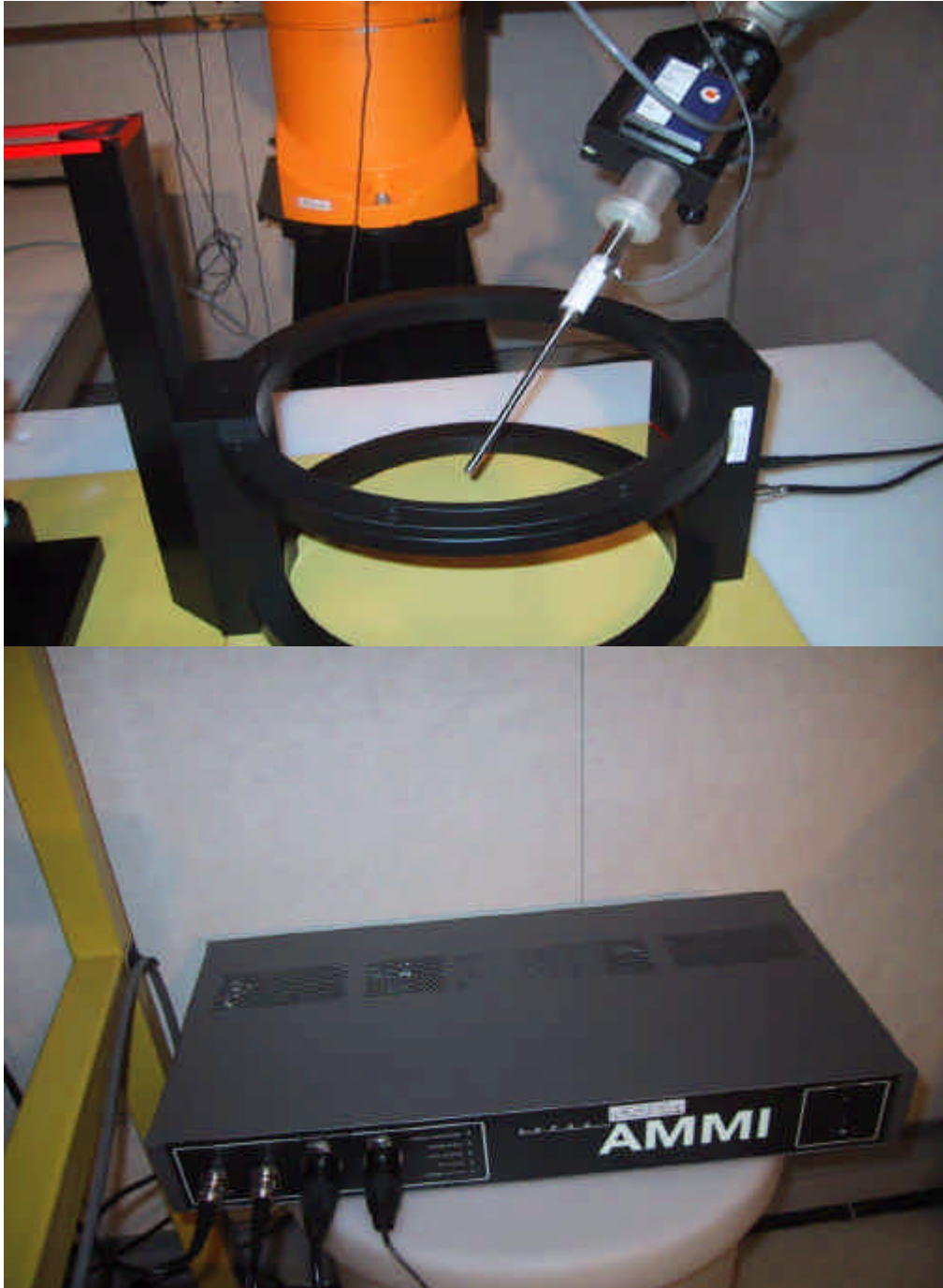
Figure E2: Probe calibration and reference signal measurement setup
