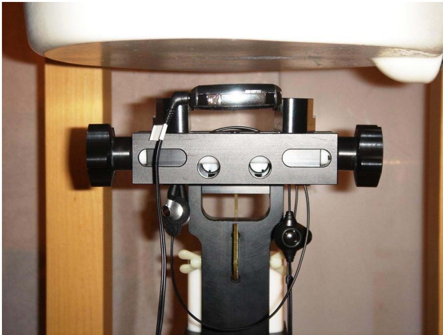
Figure E13. Body-worn configuration (No Holster, 15 mm away, with Stereo Headset and Bluetooth connected, back facing phantom)
