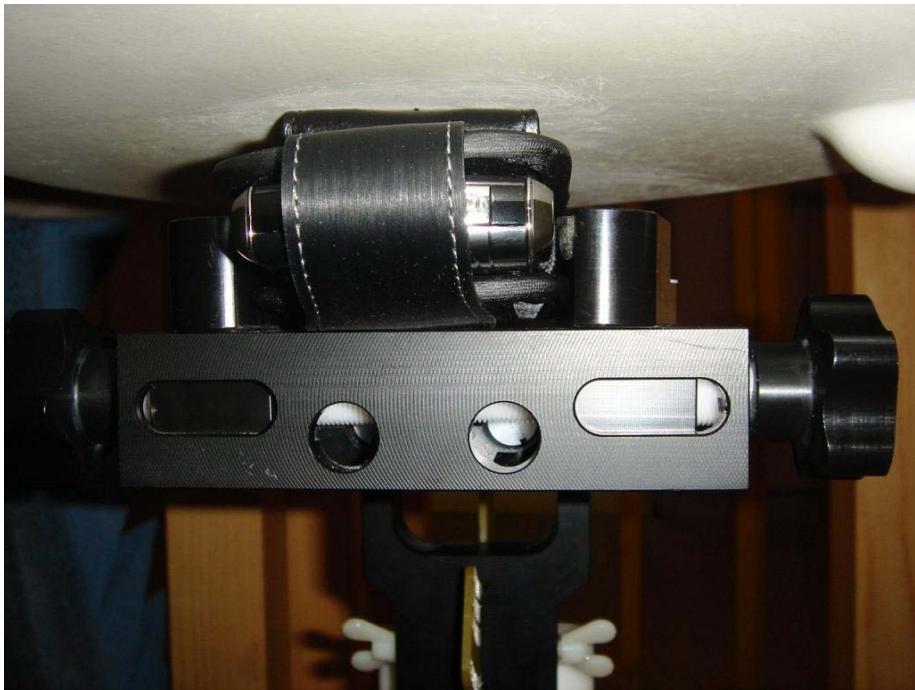
Figure E7. Body-worn configuration (Leather Holster, front facing phantom)
