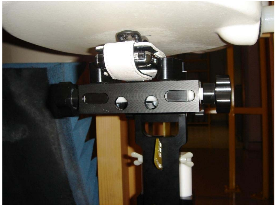
Figure E9. Body-worn configuration (Leather Swivel Holster, front facing phantom)
