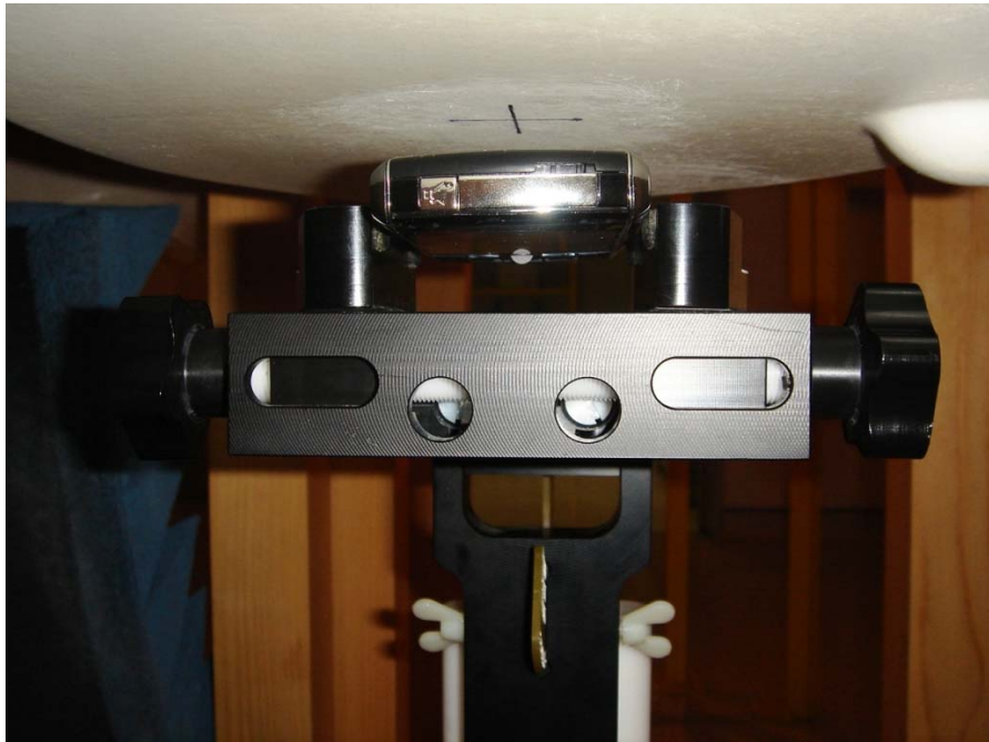
Figure E11. Body-worn configuration (No Holster, 15 mm away, back facing phantom)
