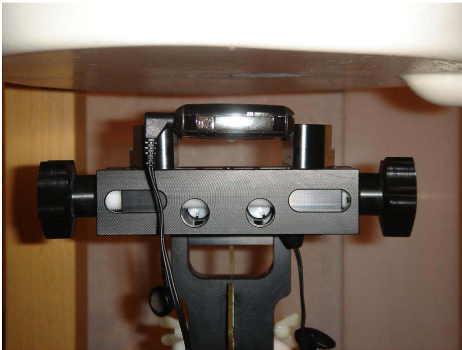
Figure E12. Body-worn configuration (No Holster, 15 mm away, with Mono Headset and Bluetooth connected, back facing phantom)
