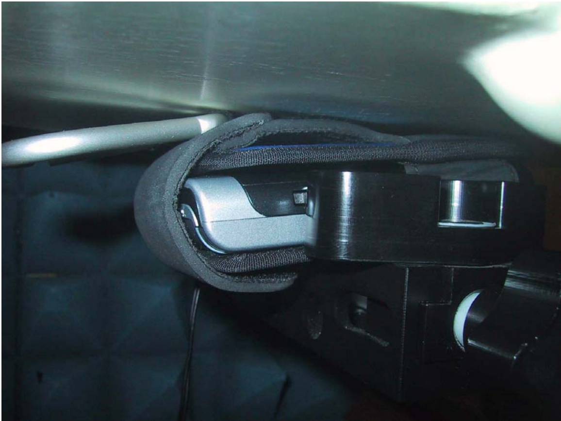
Figure E10. Body worn configuration with BT ON and headset attached (Holster 1)
