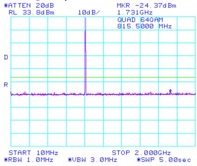
Figure 88: Spurious Conducted Emissions 2.1051
