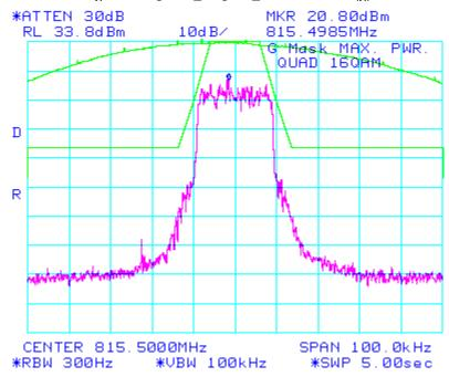
Figure 60: QUAD 16QAM G Mask 90.210(g)
