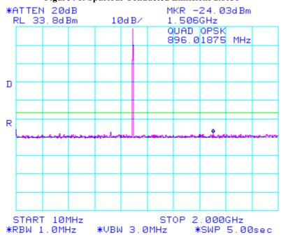
Figure 92: Spurious Conducted Emissions 2.1051
