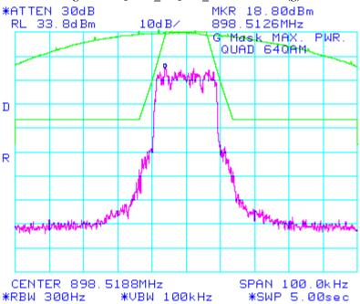
Figure 72: QUAD\_64QAM\_G Mask 90.210(g)
