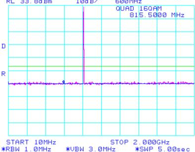
Figure 82: Spurious Conducted Emissions 2.1051
