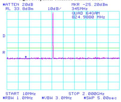
Figure 90: Spurious Conducted Emissions 2.1051
