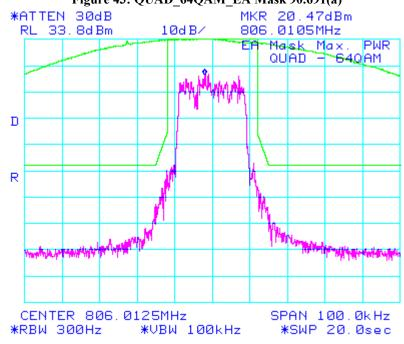
Figure 44: QUAD\_64QAM\_EA Mask 90.691(a)
