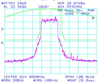
Figure 40: QUAD\_16QAM\_EA Mask 90.691(a)
