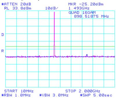
Figure 100: Spurious Conducted Emissions 2.1051
