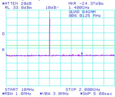
Figure 86: Spurious Conducted Emissions 2.1051
