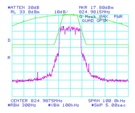
Figure 58: QUAD\_QPSK\_G Mask 90.210(g)
