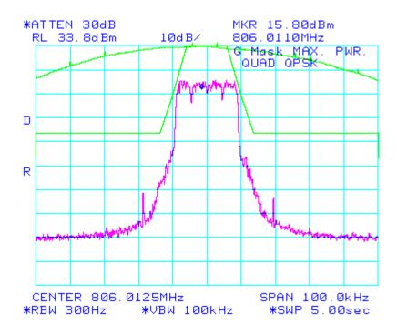
Figure 56: QUAD\_QPSK\_G Mask 90.210(g)
