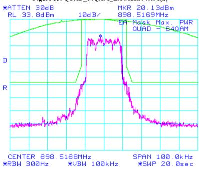
Figure 54: QUAD\_64QAM\_EA Mask 90.691(a)
