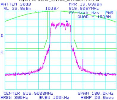
Figure 42: QUAD\_16QAM\_EA Mask 90.691(a)
