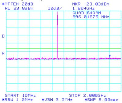
Figure 104: Spurious Conducted Emissions 2.1051
