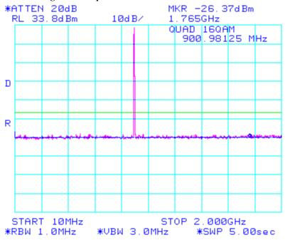
Figure 102: Spurious Conducted Emissions 2.1051
