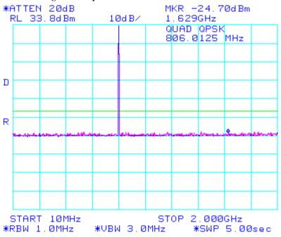
Figure 74: Spurious Conducted Emissions 2.1051
