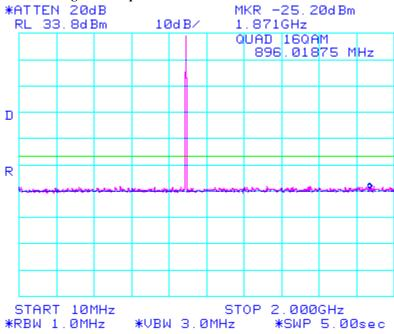
Figure 98: Spurious Conducted Emissions 2.1051
