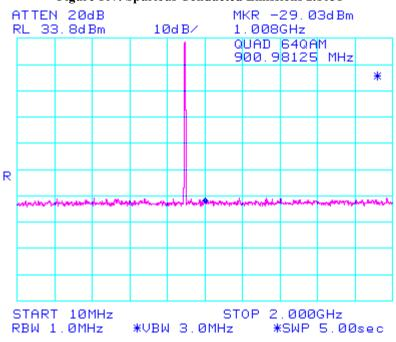
Figure 108: Spurious Conducted Emissions 2.1051
