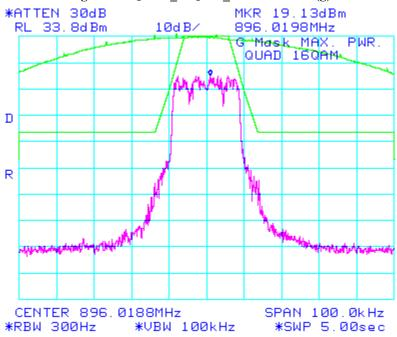
Figure 68: QUAD\_16QAM\_G Mask 90.210(g)
