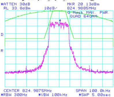
Figure 64: QUAD\_QPSK\_G Mask 90.210(g)
