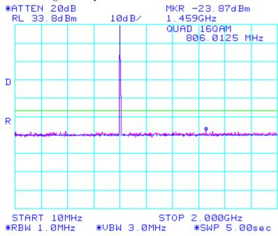
Figure 80: Spurious Conducted Emissions 2.1051
