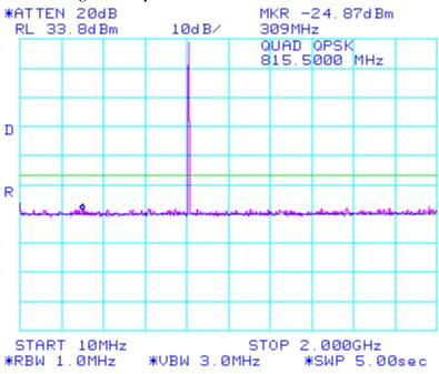
Figure 76: Spurious Conducted Emissions 2.1051
