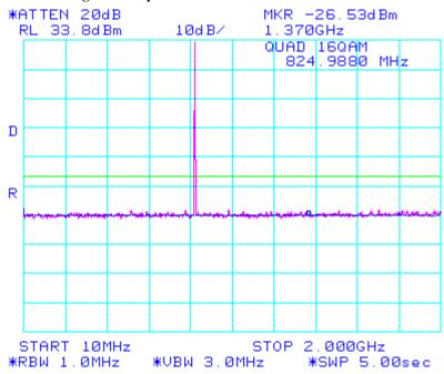
Figure 84: Spurious Conducted Emissions 2.1051
