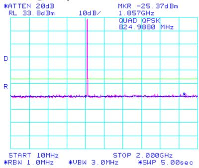
Figure 78: Spurious Conducted Emissions 2.1051
