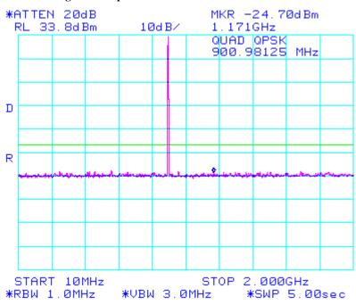
Figure 96: Spurious Conducted Emissions 2.1051
