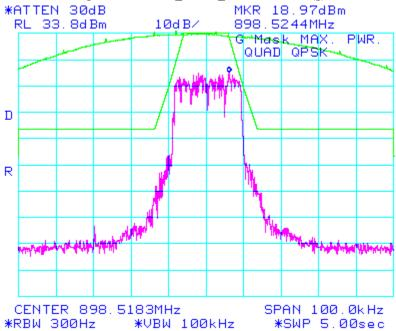
Figure 66: QUAD\_QPSK\_G Mask 90.210(g)
