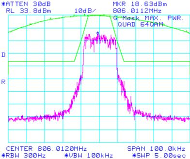
Figure 62: QUAD\_64QAM\_G Mask 90.210(g)
