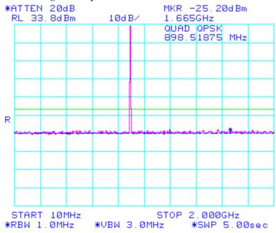
Figure 94: Spurious Conducted Emissions 2.1051
