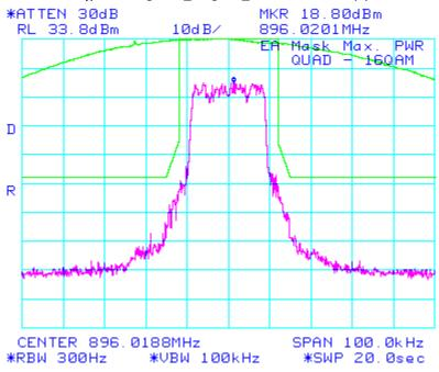
Figure 50: QUAD\_16QAM\_EA Mask 90.691(a)
