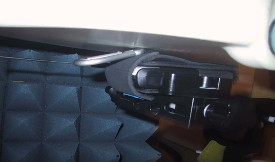
Figure E5. Body worn configuration with keychain holster (Handheld back side towards phantom)
