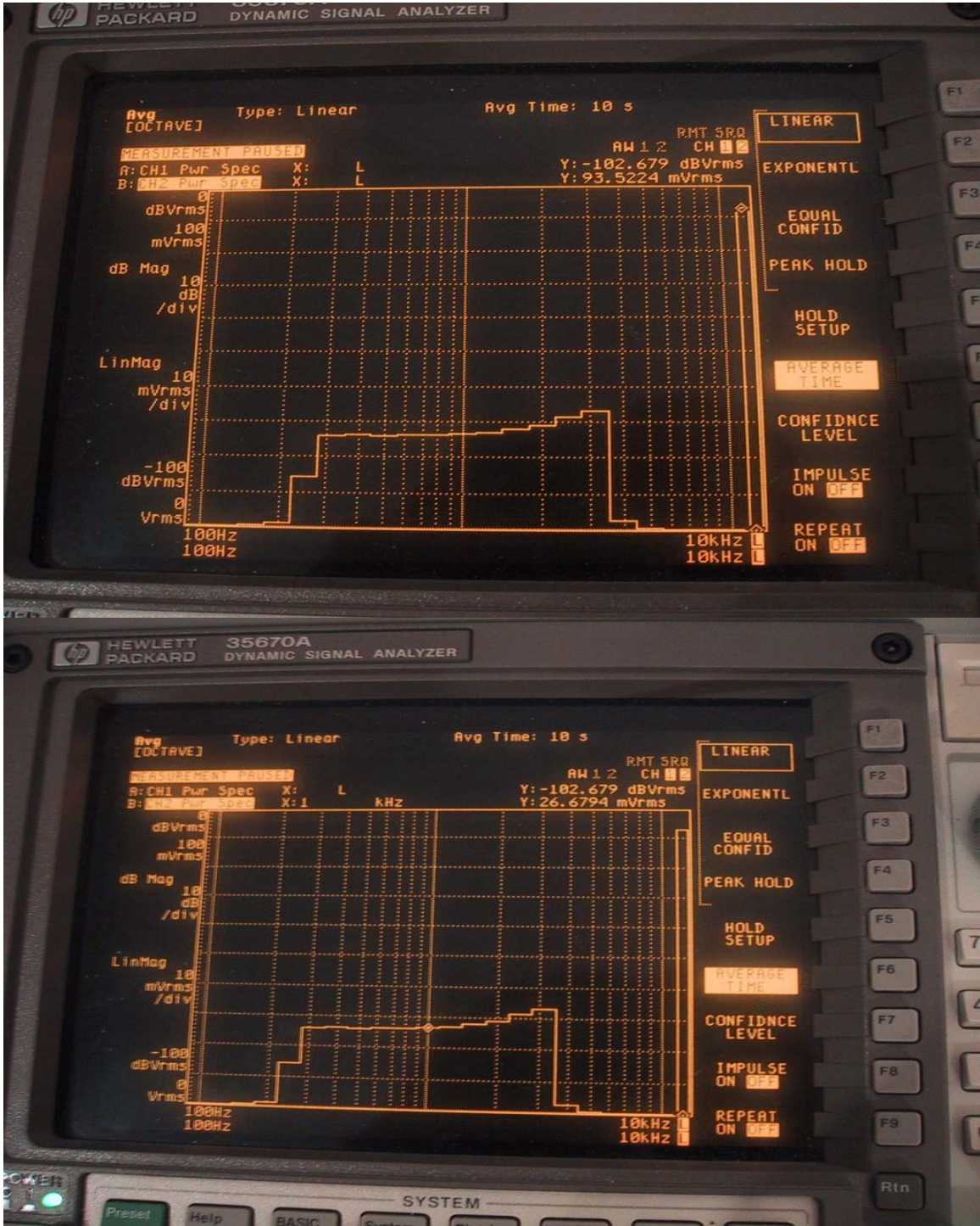
Figure 2: Top plot shows RMS time averaging power for the “48k_voice_300-3000” signal (sum of third-octave filters from 100 Hz to 10 Hz) and bottom plot is RMS power at 1 kHz third-octave filter.
