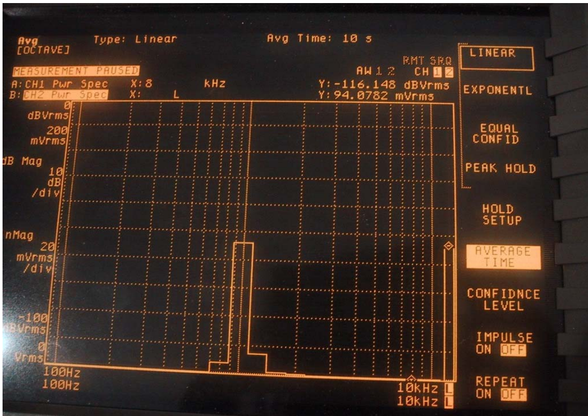
Input level measurement analyzer plots for the sinusoidal 1.025 kHz signal
