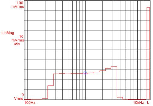
Top plot shows RMS time averaging voltage (sum of third-octave filters from 100 Hz to 10 Hz) and bottom plots is RMS voltage at 1 kHz third-octave filter.
