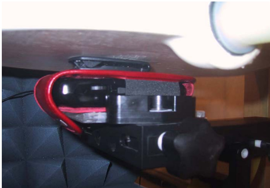
Figure E8. Body worn configuration, LeatherSwivel holster
