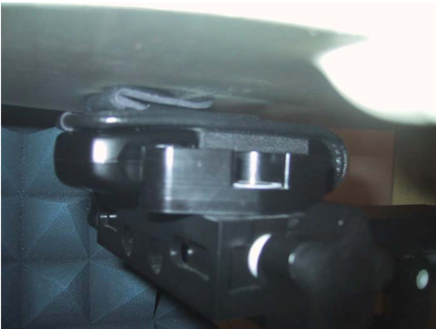
Figure E6. Body worn configuration, leather holster
