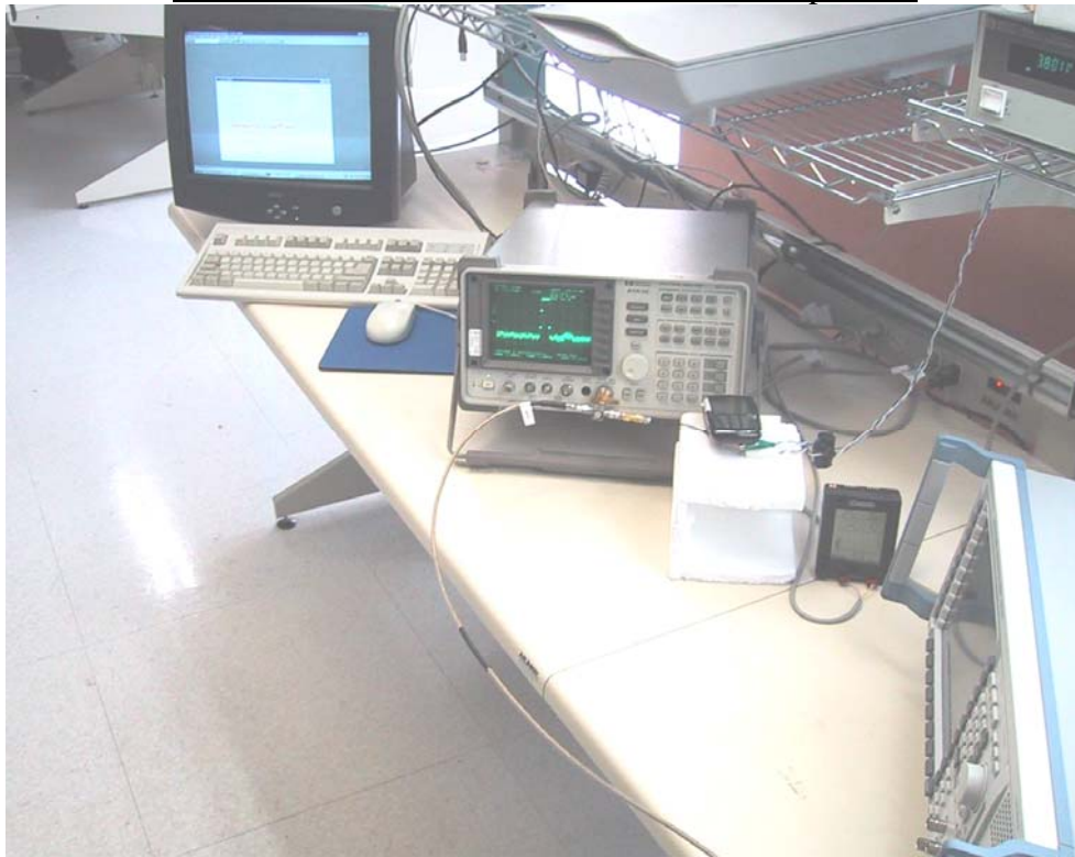
RF Conducted Bluetooth Emission Test-Setup Photo
