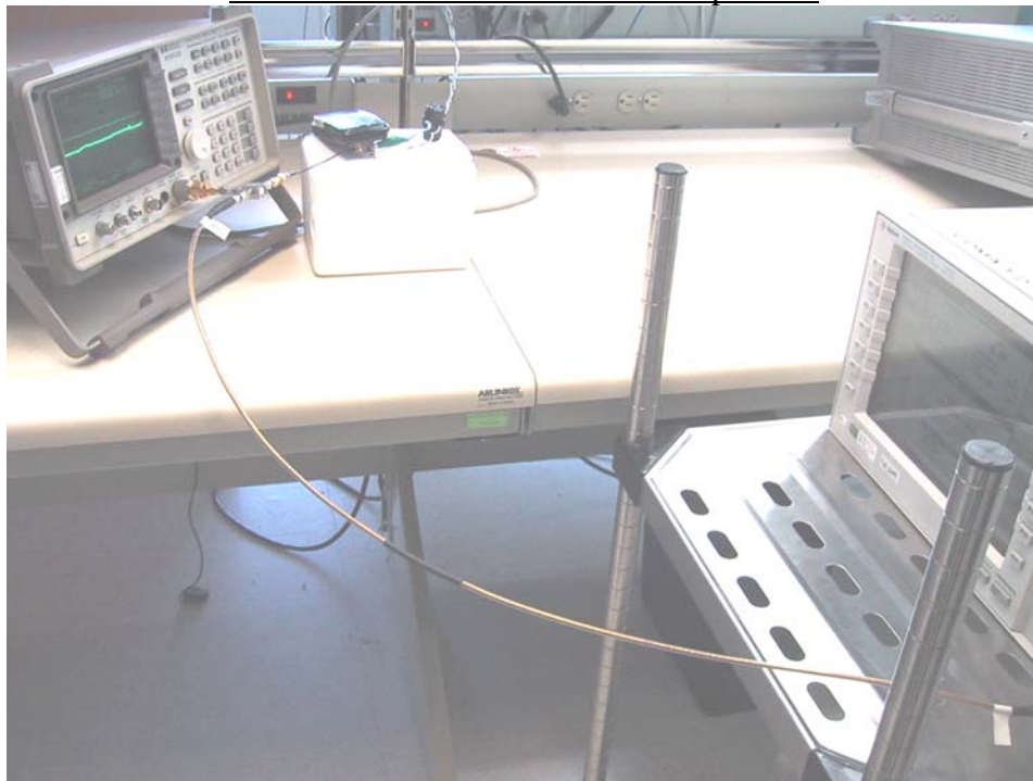
RF Conducted Emission Test-Setup Photo
