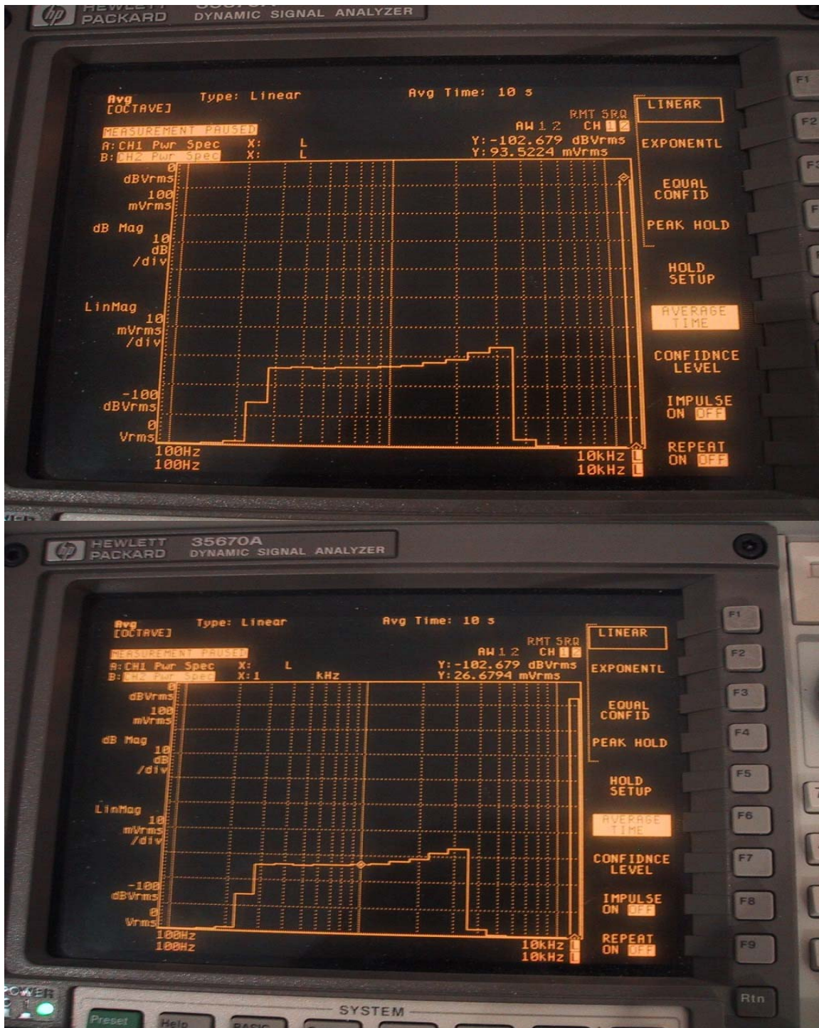
Figure 2: Top plot shows RMS time averaging power for the “48k_voice_300-3000” signal (sum of third-octave filters from 100 Hz to 10 Hz) and bottom plot is RMS power at 1 kHz third-octave filter.
