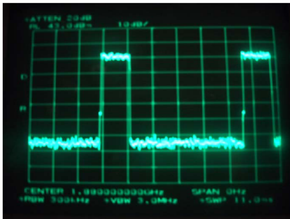
0 Hz Span CDMA 1/8 Gating Plot (1880MHz)
