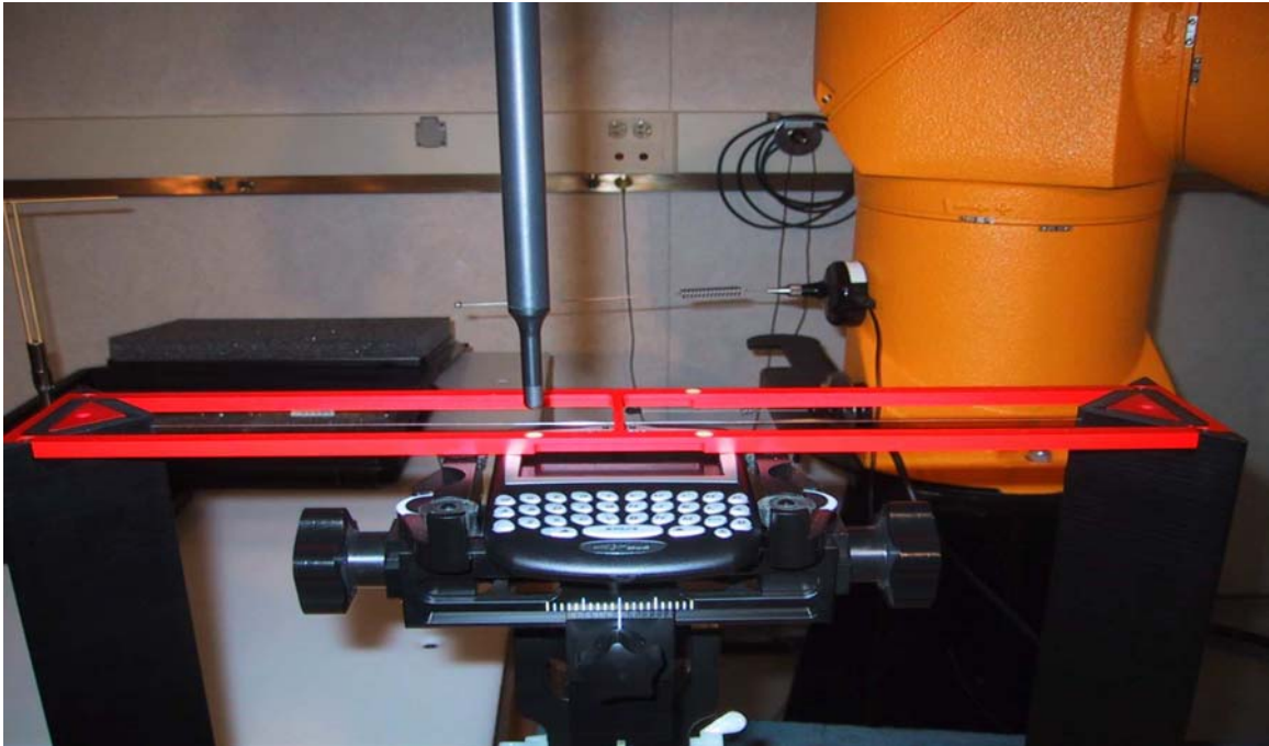
Figure 6 – HAC RF emission H-field test setup
