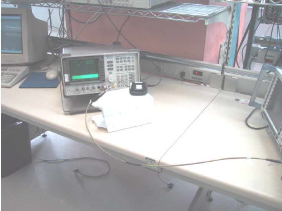
RF Bluetooth Conducted Emissions Test-Setup Photo for FCC CFR 47 Part 15, Subpart C, Class B
