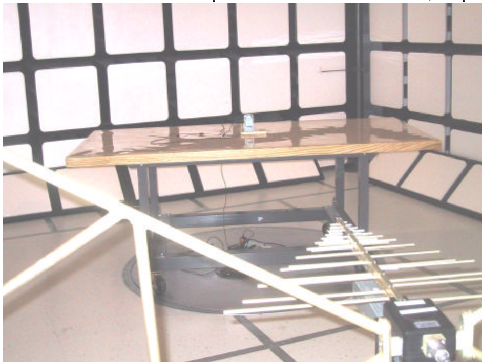
Radiated Emissions at 3 metres Test-Set-up Photo for FCC CFR 47 Part 15, Subpart B, Class B
