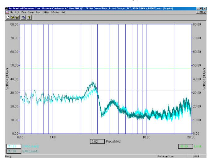
The Travel Charger was connected to the Handheld in battery charge mode. The ac input to the Travel Charger was 120 volts, 60 Hz.
