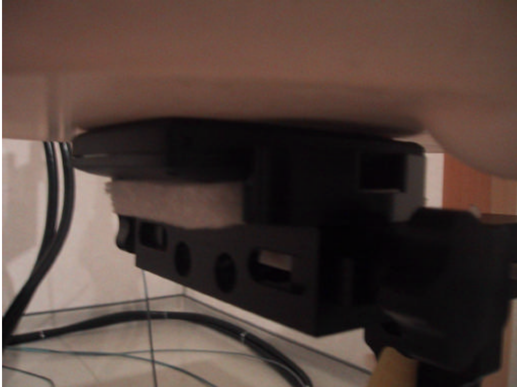
Figure E2. Body worn with back side of handheld touching flat phantom for inside shirt pocket configuration
