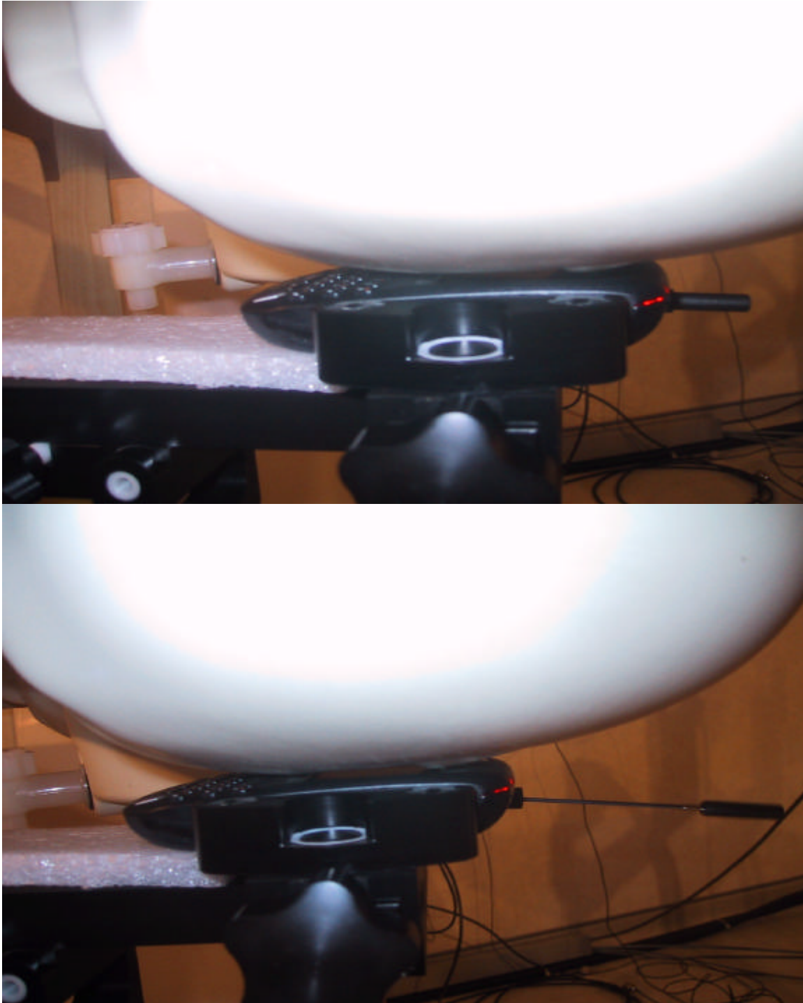
Figure E1. Left ear touch configuration
