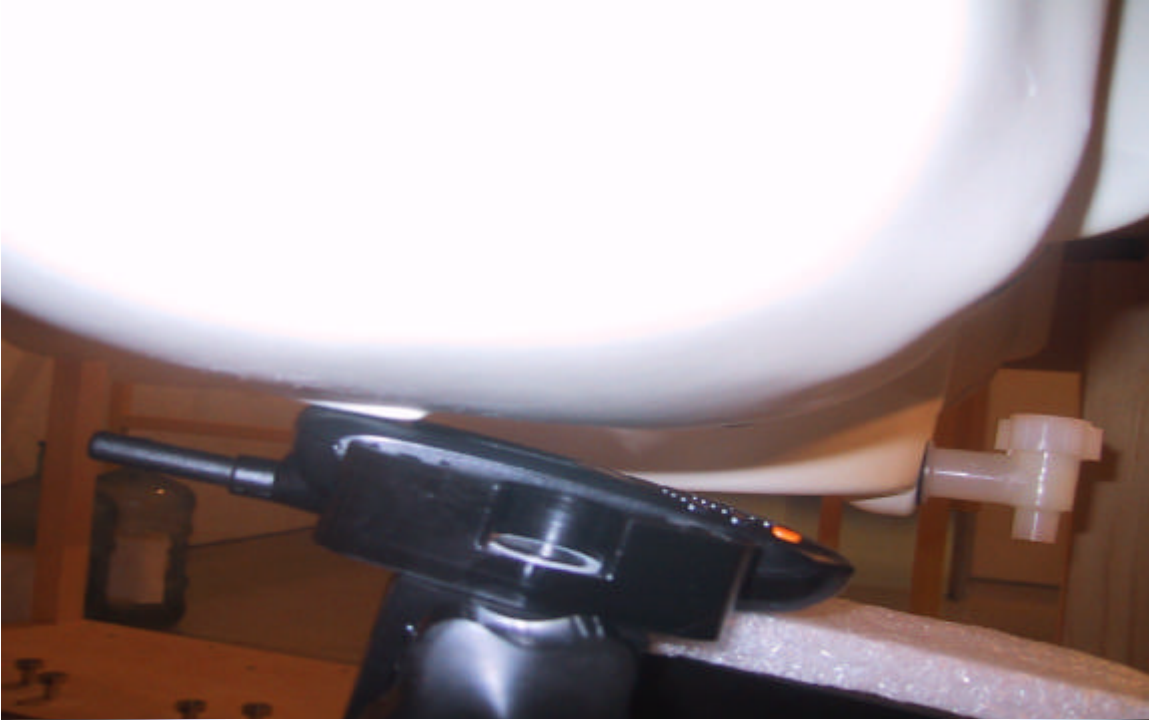
Figure E3. Right ear touch configuration
