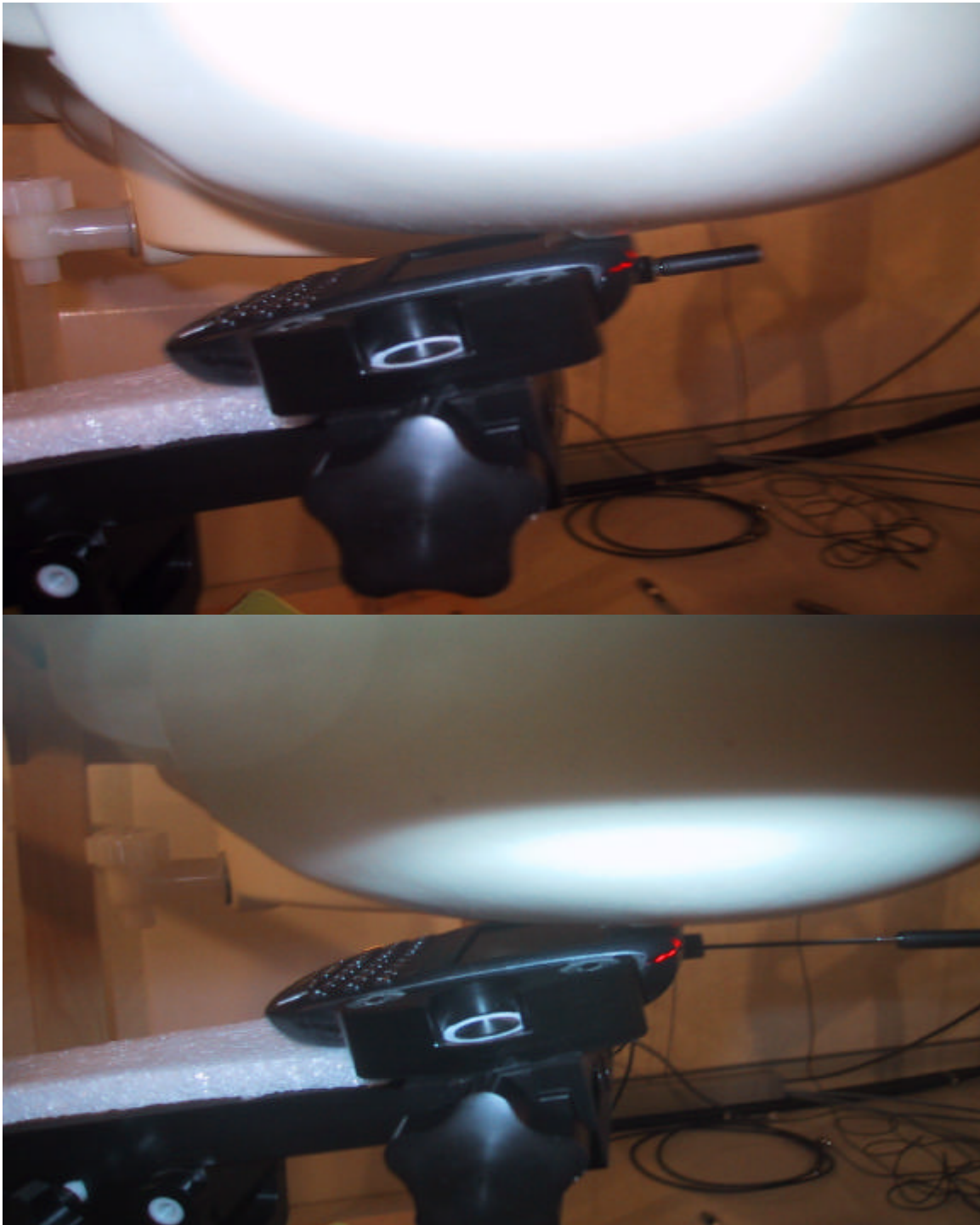
Figure E2. Left ear tilted configuration
