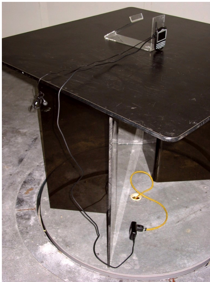
Radiated Emissions Measurement in Open Area Test Site Testing setup: BlackBerry RAL10IN connected to charger and earphone
