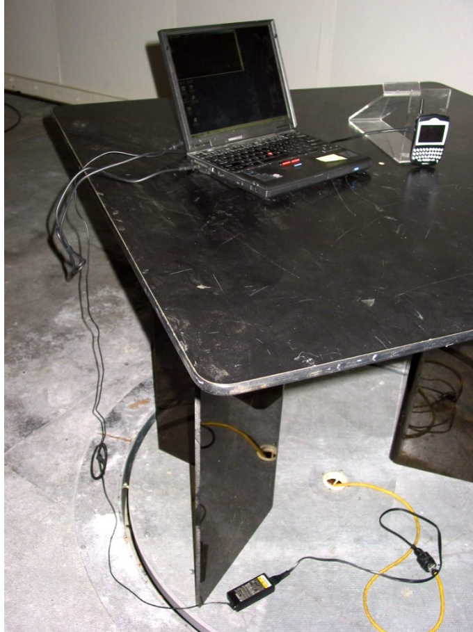
Radiated Emissions Measurement in Open Area Test Site Testing setup: BlackBerry RAL10IN connected to laptop PC
