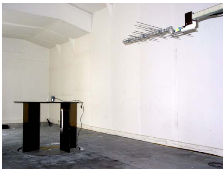
Radiated Emissions Measurement in Open Area Test Site (Frequency range: 200 MHz – 960 MHz) Configuration: BlackBerry RAL10IN connected to charger and earphone
