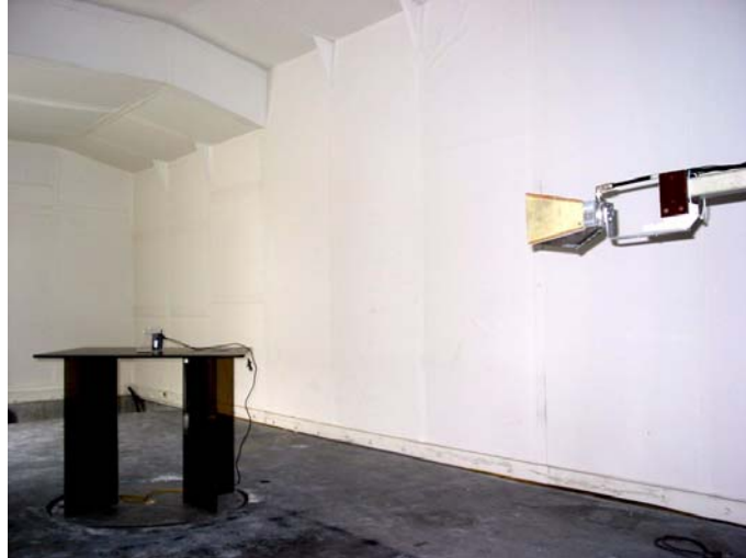
RIM RAL10IN BlackBerry Wireless Handheld tested for Spurious Emissions from Transmitter Frequency Range: 1 GHz – 18 GHz
