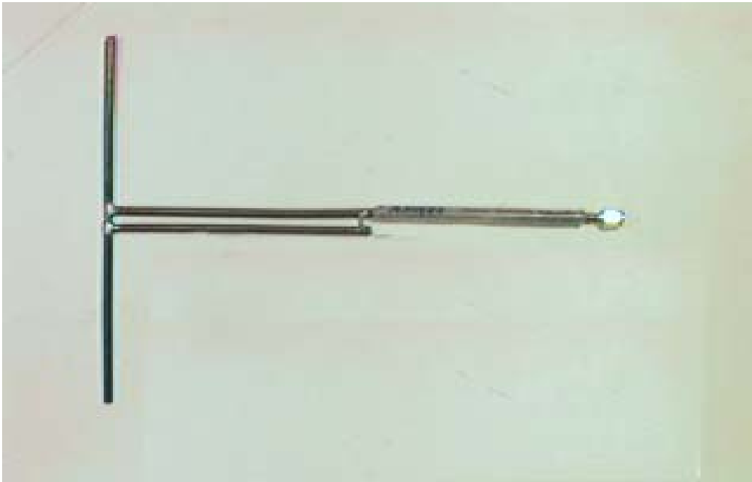
Reference Dipole Antenna Used for ERP Measurement
