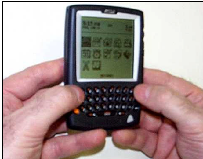
Figure 4. Experienced user typing with two thumbs holds Proton pager near the bottom of the device
