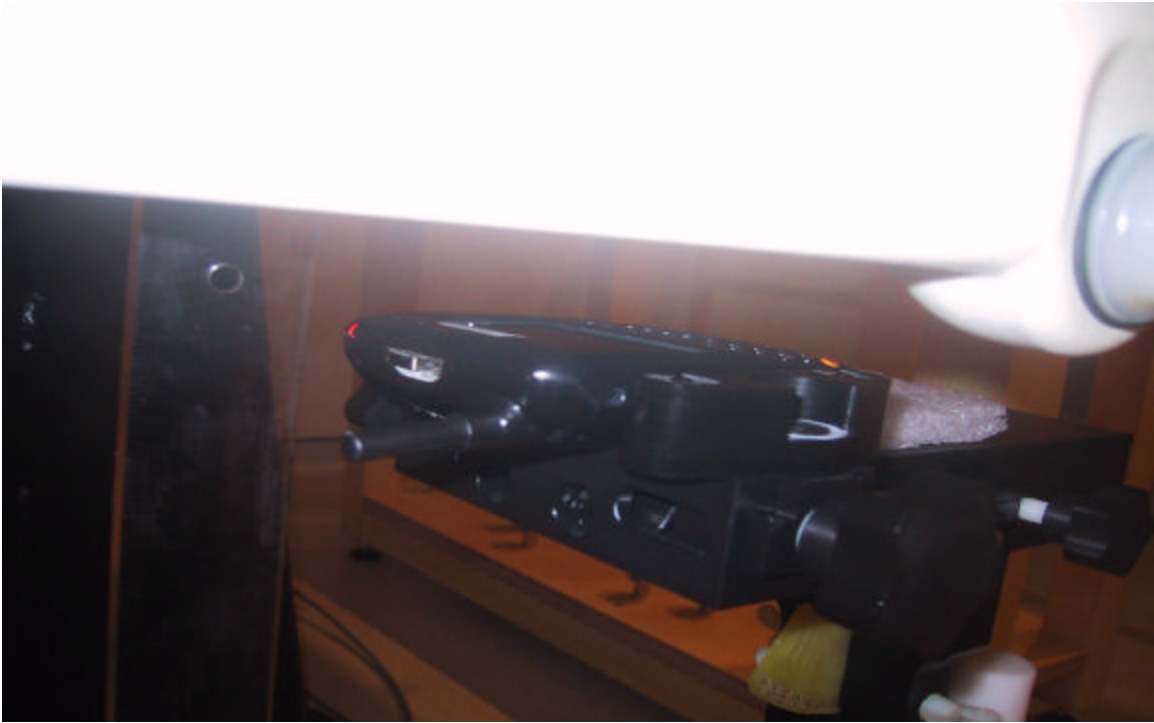
Figure B1. Face SAR with 2.5 cm separation distance, retracted antenna
