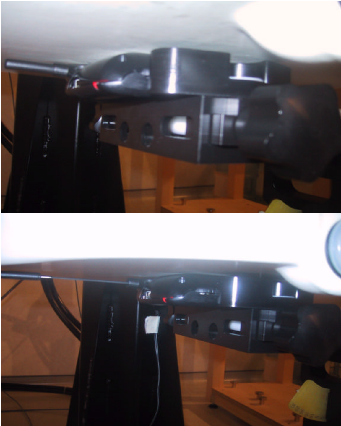
Figure C8. Hand SAR configuration, unit back touching flat phantom
