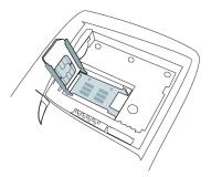
Inserting the SIM card
