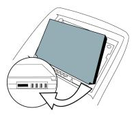
Aligning the battery connectors
